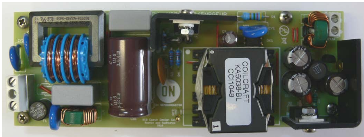
Figure 26. Photograph of the Designed Prototype (Real Dimensions are 146.6 x 50.8 mm)
