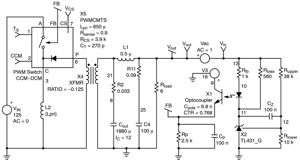
**Figure 10. The NCP1351 Model in a Flyback Converter**
