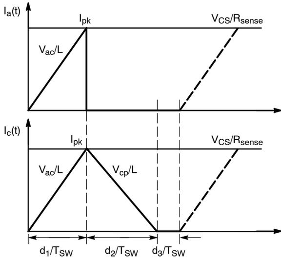
Figure 4. The Current Waveforms in DCM:  $I_a$ ,  $I_c$
