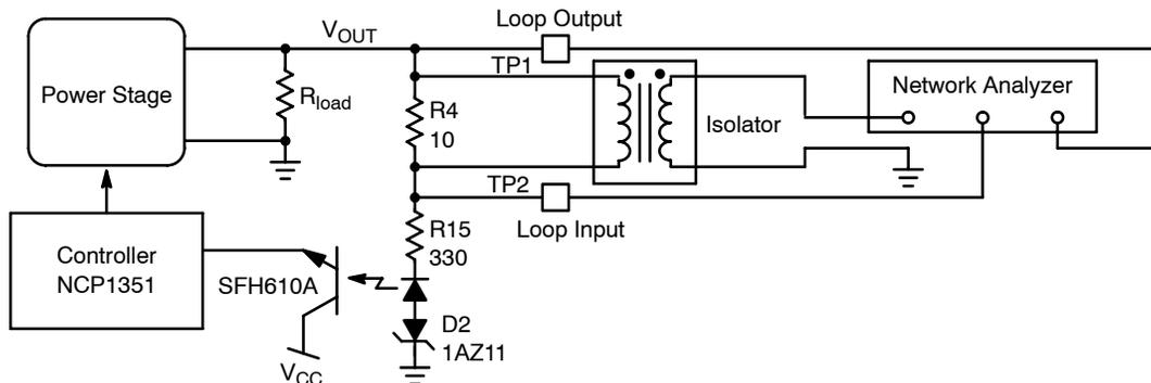
**Figure 15. Loop Response Measurement Principle**
