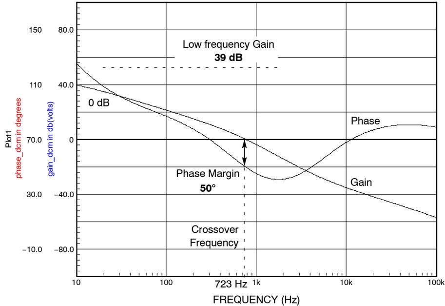
**Figure 19. Measured Loop Response in DCM**
