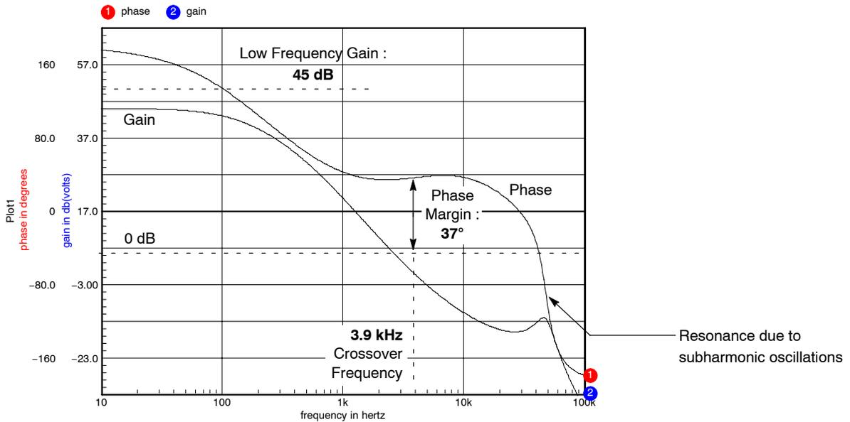
Figure 17. Simulated Loop Response in CCM
