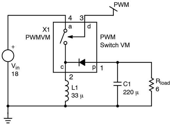
Figure 3. PWM Switch in the Buck-boost Converter
