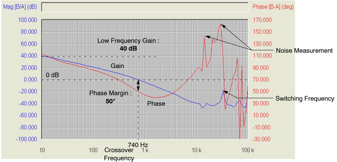
**Figure 18. Measured Loop Response in CCM**
