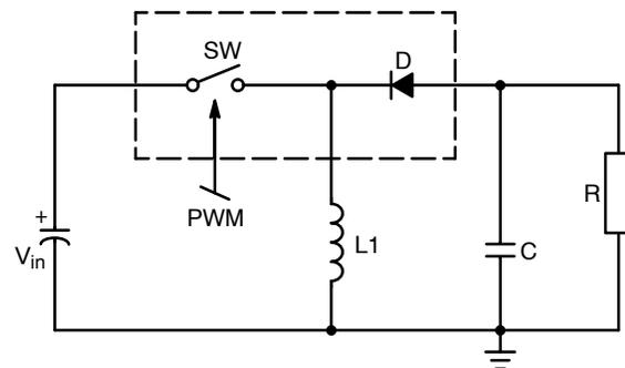
Figure 2. Buck-Boost Converter
