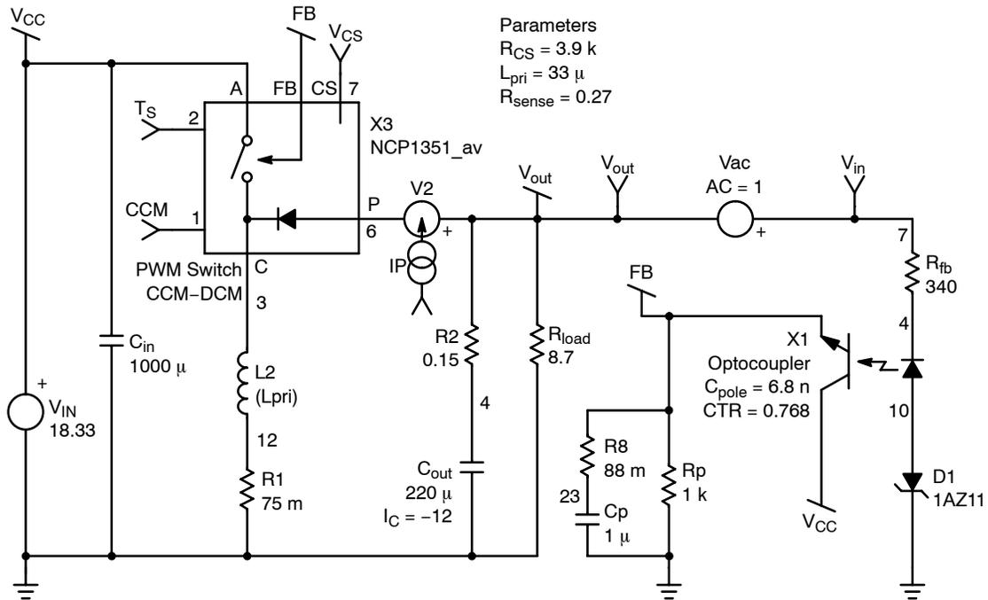
**Figure 12. The Buck-boost Model Implemented in SPICE**
