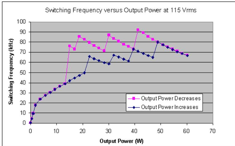
Figure 11. Switching Frequency Evolution versus Output Power at  $V_{in} = 115$  Vrms
