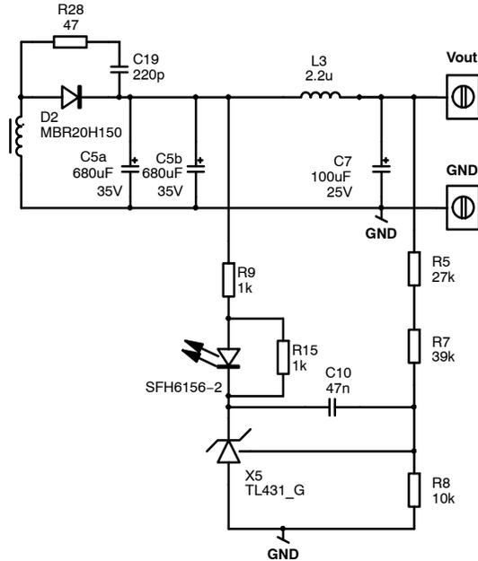
**Figure 4. TL431 Biased by a 1 kΩ Resistor**
