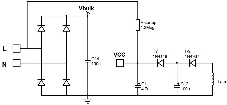
**Figure 6. The Startup Resistor is Connected to the Half-Wave**
