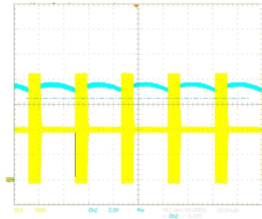
Figure 22. Operation in the Skip Mode
