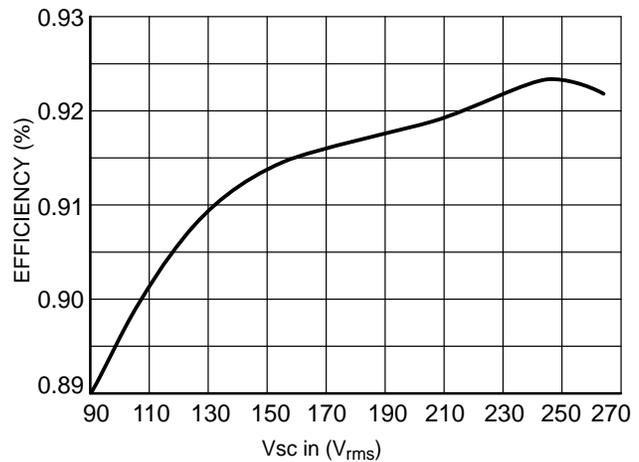
**Figure 12. Efficiency of the Example Converter versus Input Voltage for Full Loaded Output**
