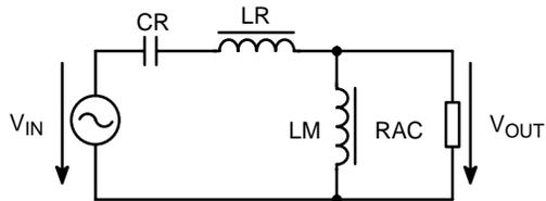
**Figure 5. Substitutive Schematic of the LLC Resonant Converter**
