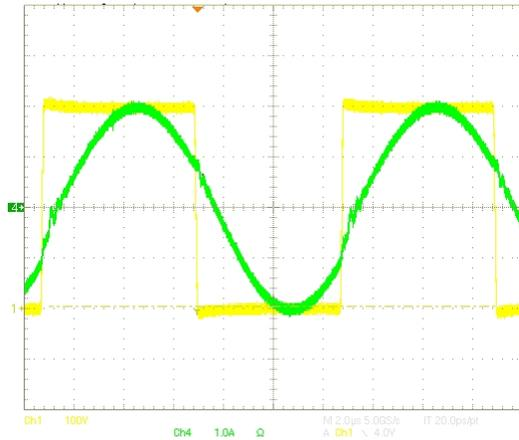
Figure 14. Primary Current and Waveforms for Full Loaded Converter
