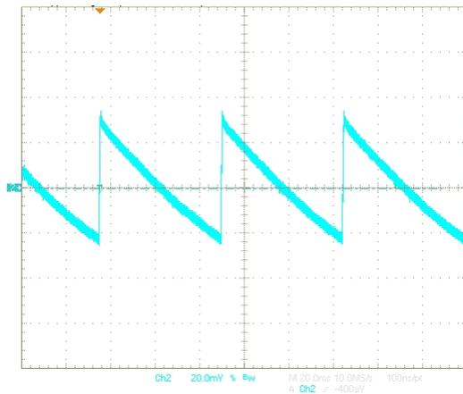
Figure 19. Output Ripple During the Skip Mode
