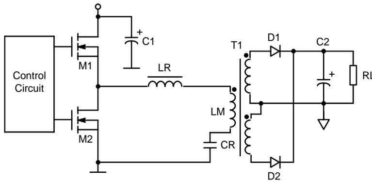
**Figure 4. Power Stage of the LLC Resonant Converter**
