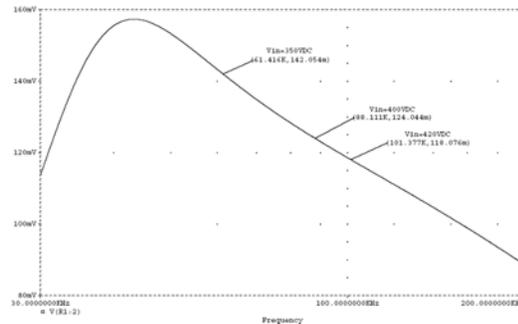
Figure 10. Simulated Gain Characteristic of Proposed LLC Converter – Full Load Conditions
