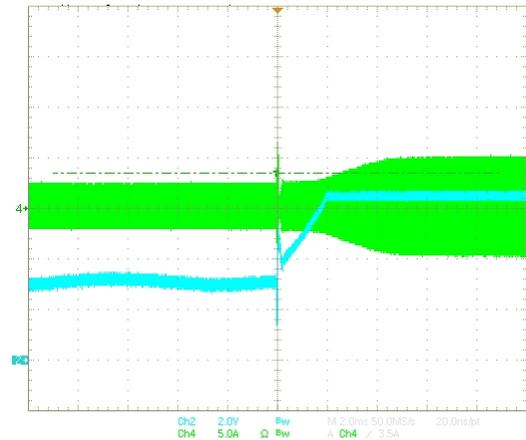
Figure 21. Full Load to Short Circuit Transition
