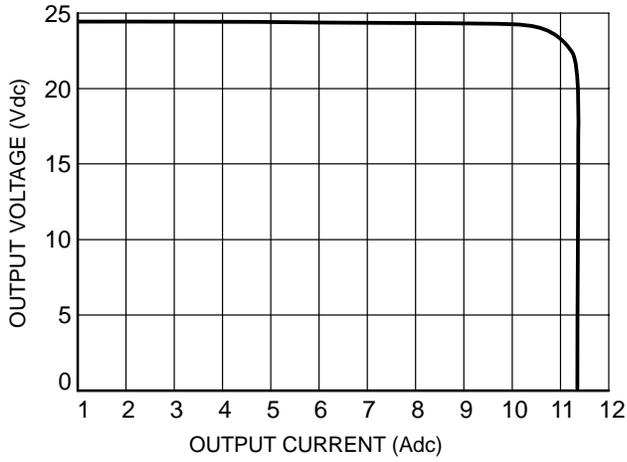
Figure 13. Loading Characteristic of the Proposed Converter
