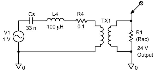
Figure 9. Simulation Schematic of the Proposed Converter
