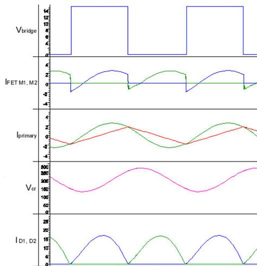
Figure 8. Typical waveforms of the LLC converter operating in the 2<sup>nd</sup> area of the gain characteristic.
