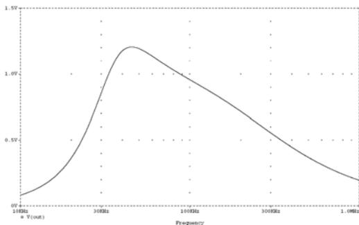
Figure 6. Typical Gain Characteristic of the LLC Resonant Converter
