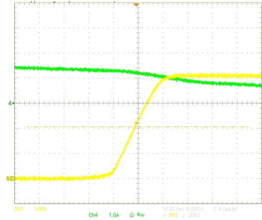
Figure 15. Detail of the ZVS Condition – Rising Edge
