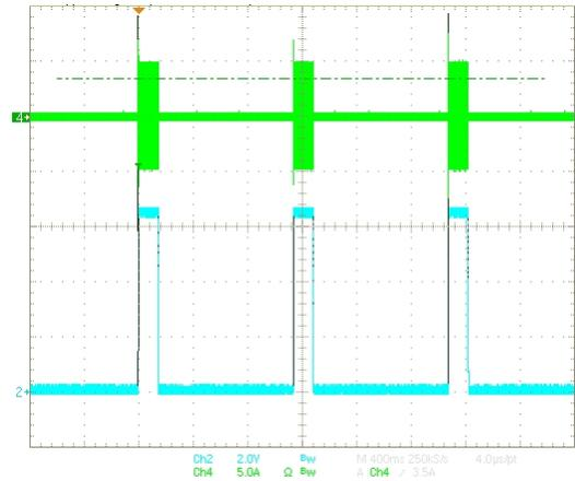
Figure 20. Operating Under Short Circuit
