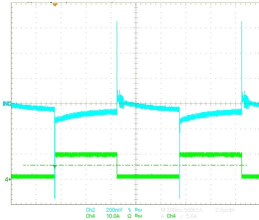
Figure 17. Load Regulation for 230 V Input Voltage
