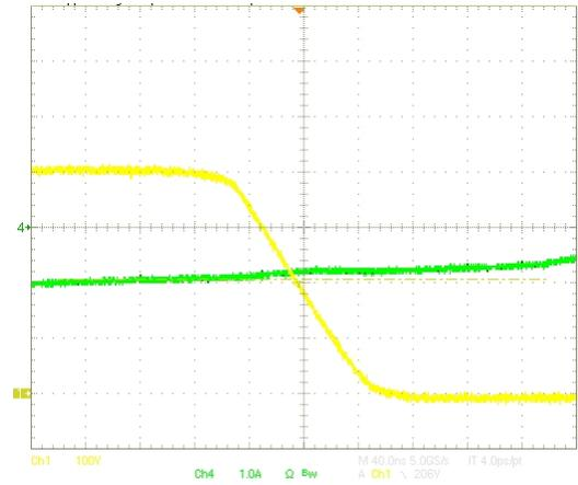
Figure 16. Detail of the ZVS Condition – Falling Edge
