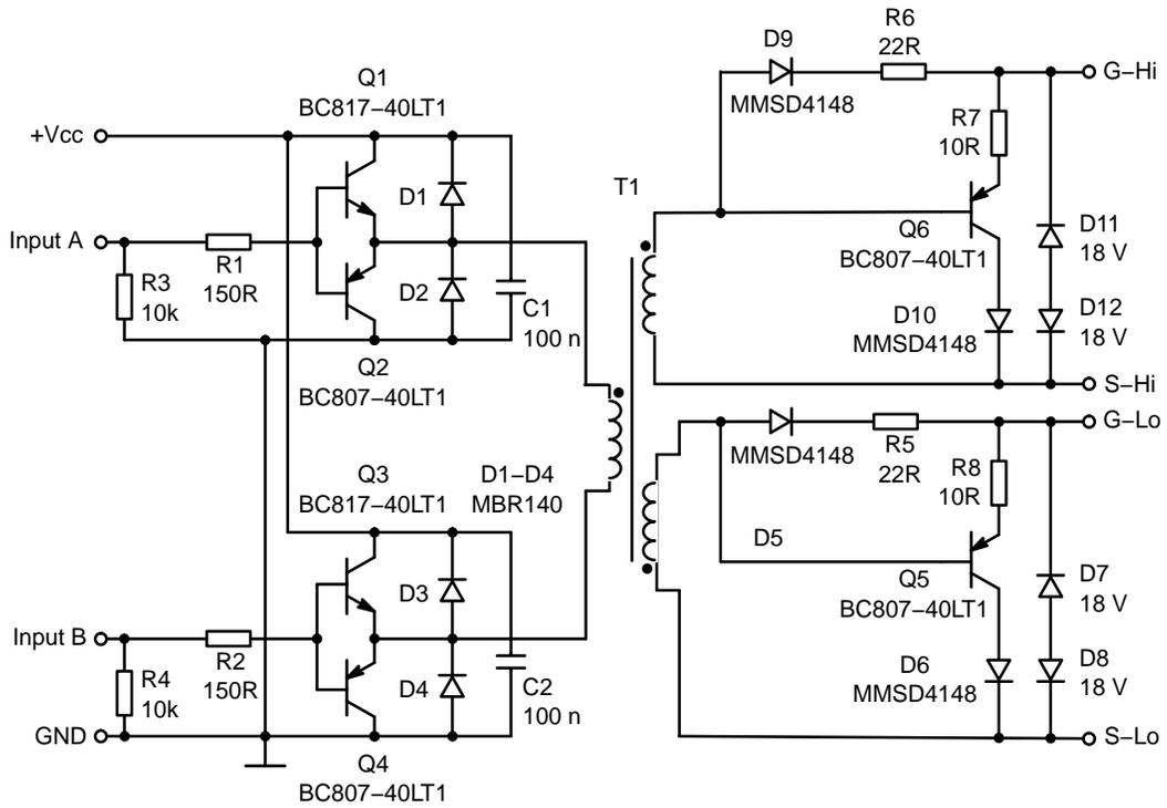
Figure 2. Connection of the MOSFET Driver with Transformer
