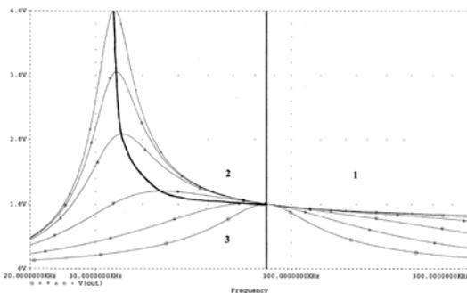
Figure 7. Couple of Gain Characteristic for Different Load Conditions
