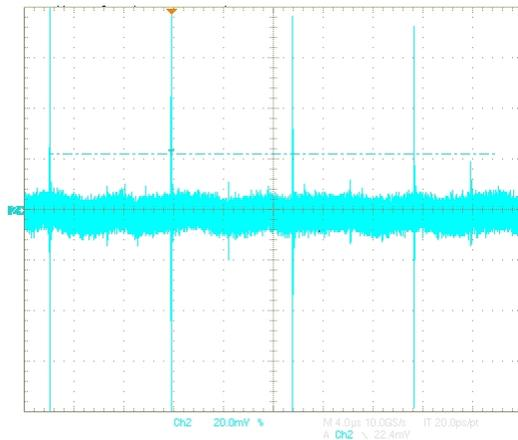
Figure 18. Output Ripple Under Full Load
