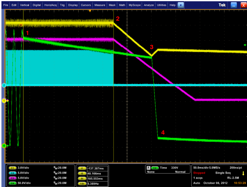
Figure 4. Active X2 Capacitor Discharge
