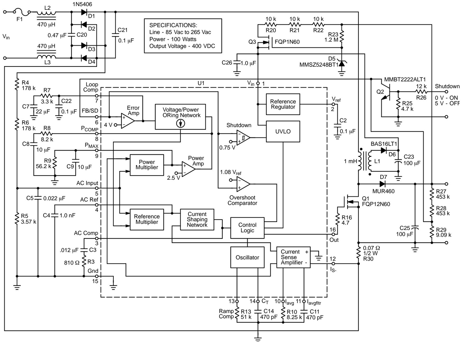
Figure 1. Applications Circuit Schematic
