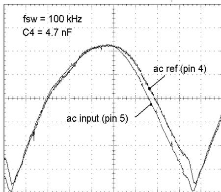
**Figure 2. AC Ref with Phase Delay**
