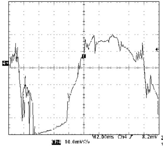
**Figure 1. Example of Input Current Waveform Distortion Due to Noise Issues**
