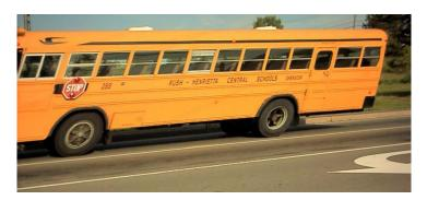
Figure 1. This Image of a Bus was taken using a CMOS Imager in Rolling Shutter Mode
