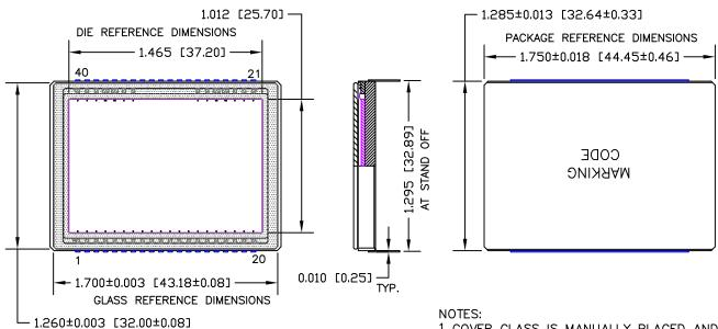
1. COVER GLASS IS MANUALLY PLACED AND VISUALLY ALIGNED OVER DIE — LOCATION ACCURACY IS NOT GUARANTEED.
