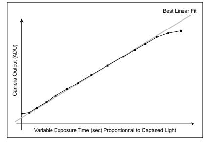
Figure 2. Detector CCD Output vs. Exposure Time
