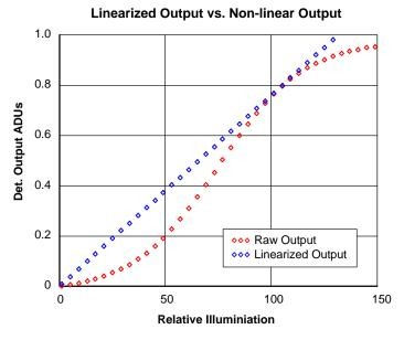
Figure 6. Non-linear Output to Be Corrected
