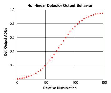
Figure 5. Simulated Non-linear CCD/Detector Output Behavior
