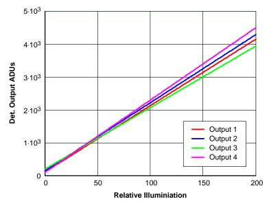
Figure 4. The 4 CCD Output Signal vs. Different Illumination Levels
