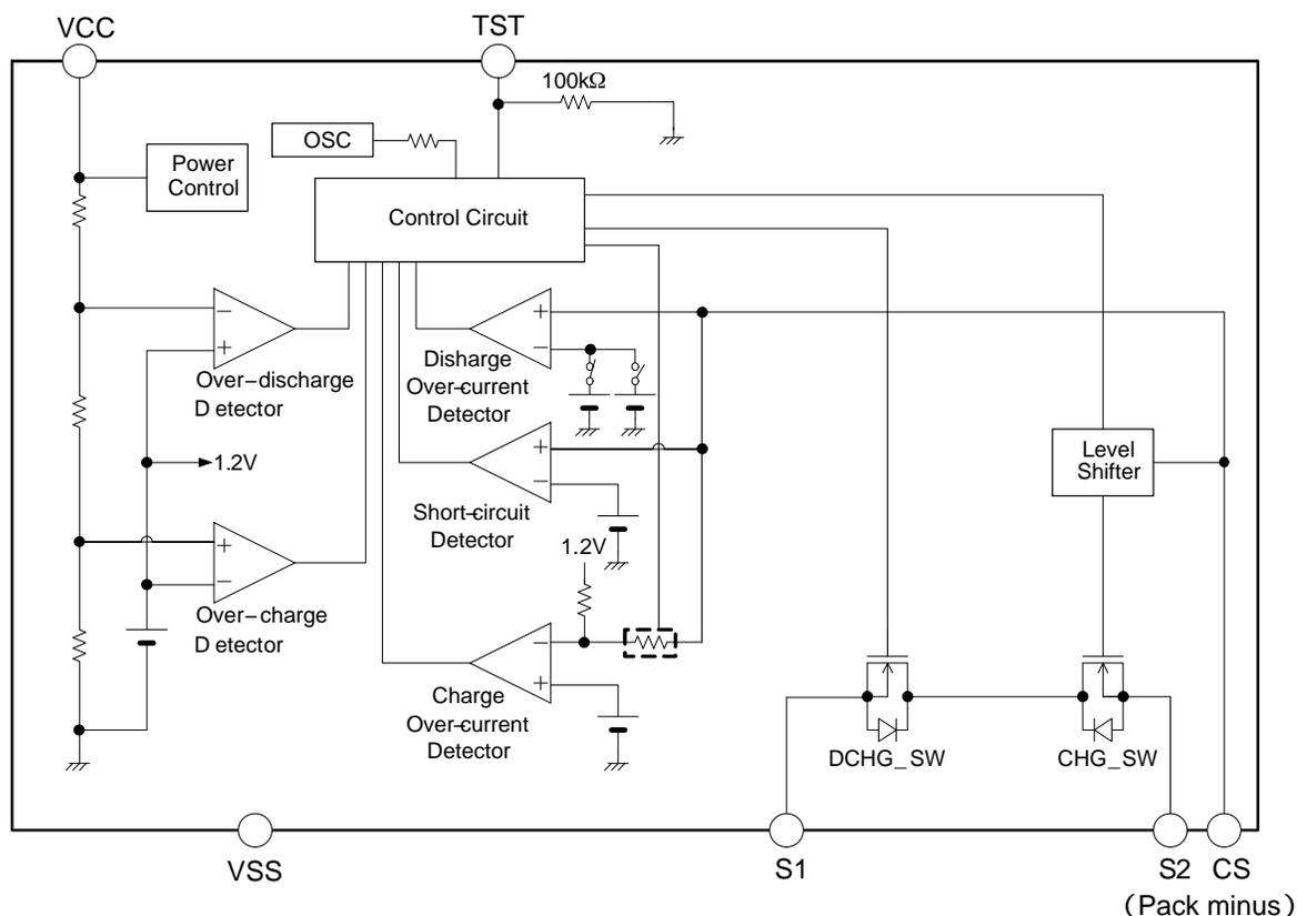
**Figure 6. Block Diagram**
