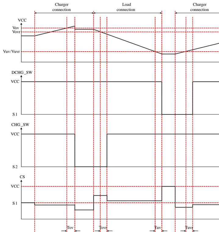
Figure 7. Over-charged detection/release, Over-discharge detection/release (Connect charger)
