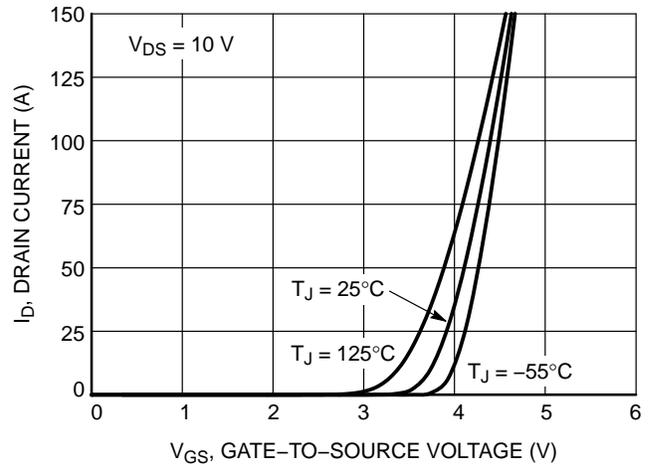
Figure 2. Transfer Characteristics
