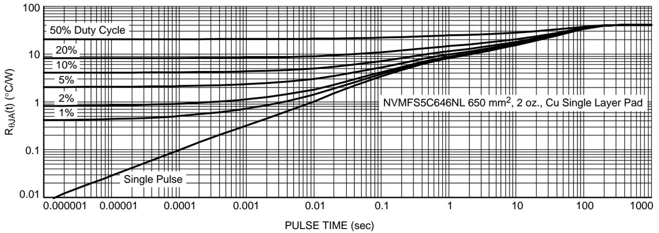
Figure 13. Thermal Characteristics
