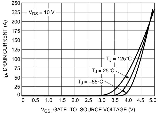
Figure 2. Transfer Characteristics
