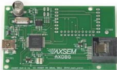
Figure 1. DVK Debug Adapter
