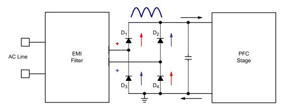
Figure 1. The Input Current Flows Through Two Diodes
