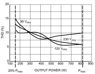
Figure 16. Total Harmonic Distortion Over the Load Range
