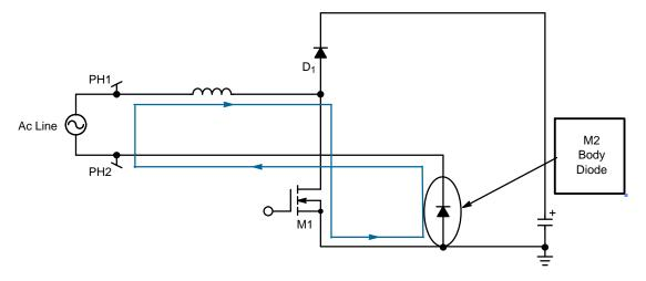
Figure 3. MOSFET Conduction Phase ("PH1" Half-Wave)
