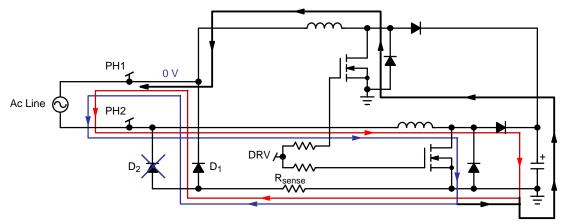
Figure 8. Operation for the "PH2" Half-Wave
