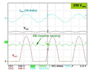
Figure 13. Typical Waveforms at Low Line (Left) and High Line (Right)
