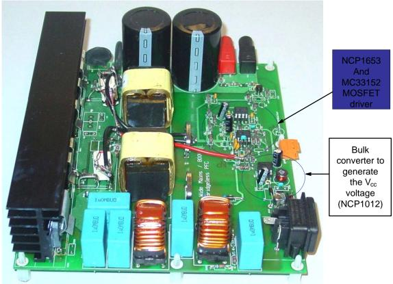
Figure 12. Photograph of the Evaluation Board
