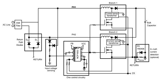
Figure 10. Simplified Application Schematic
