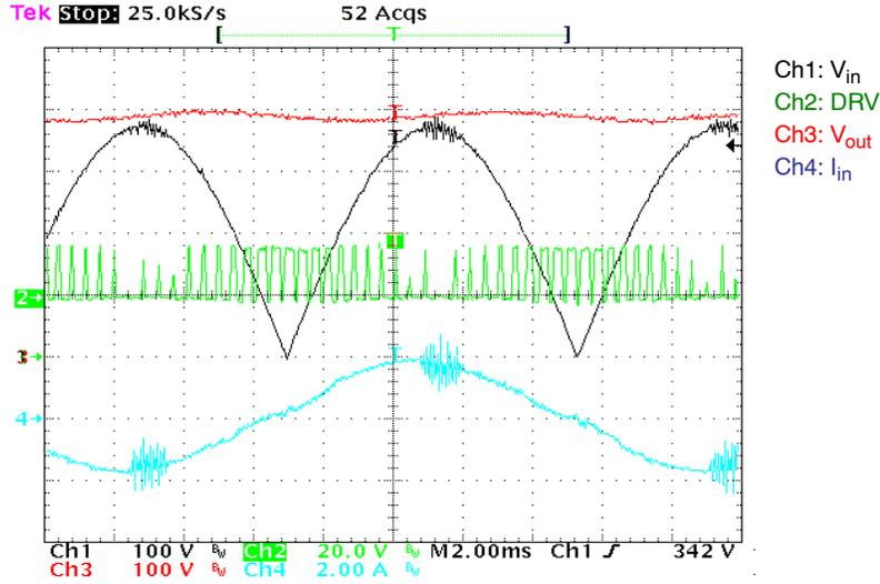
Figure 5. The Waveforms at 265 V<sub>ac</sub>, 300 W as Controlled by 200 kHz NCP1654
