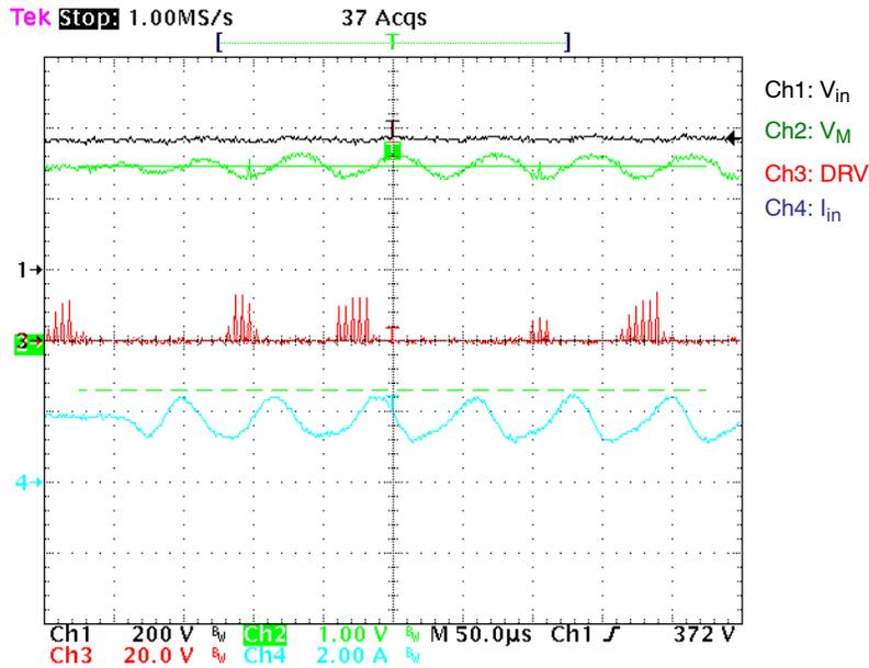
Figure 4. Zoom-in with Waveforms at Peak of 265 V<sub>ac</sub>
