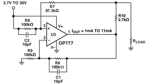
Figure 14. Single-Supply Current Source
