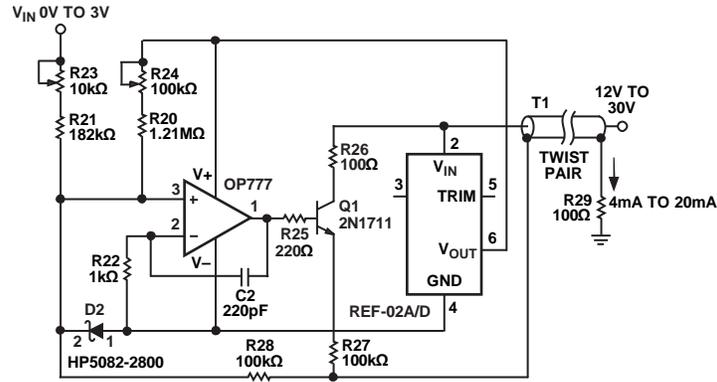
Figure 2. Self-Powered 4 mA to 20 mA Current Loop Transmitter
