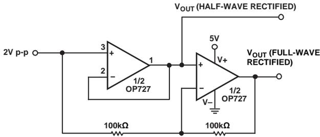
Figure 12. Single-Supply Half-Wave and Full-Wave Rectifier
