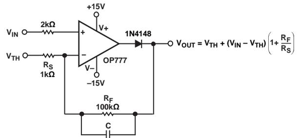
Figure 11. Precision Threshold Detector/Amplifier
