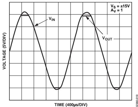
Figure 19. Input Voltage Can Exceed the Supply Voltage Without Damage
