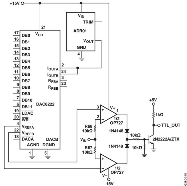
Figure 10. Programmable High Resolution Window Comparator
