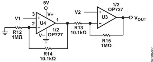
Figure 5. Single-Supply Micropower In-Amp
