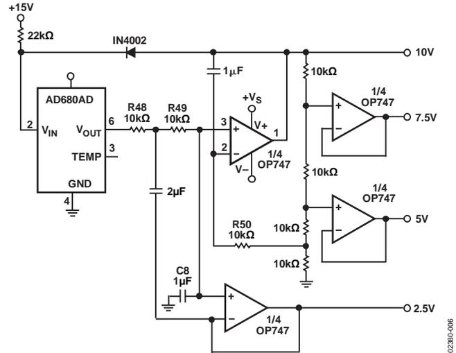
Figure 6. Multiple Output Tracking Voltage Reference
