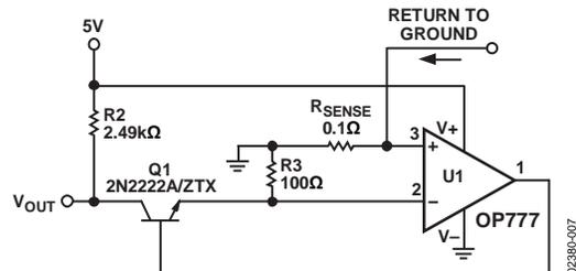
Figure 7. Low-Side Current Sensing Circuit
