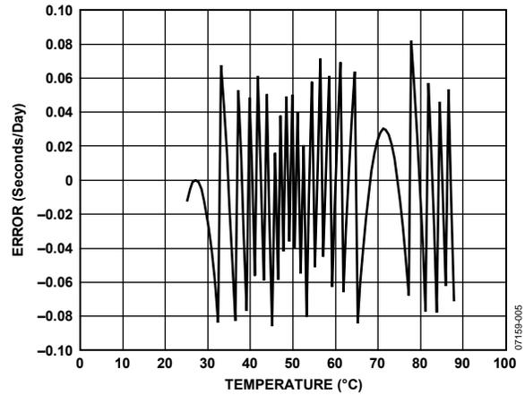
Figure 5. Sec/day Error with Temperature Compensation
