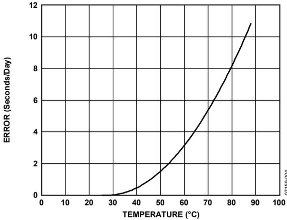
Figure 4. Sec/day Error with No Temperature Compensation
