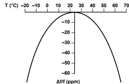
Figure 3. Parabolic Temperature Curve of a Crystal
