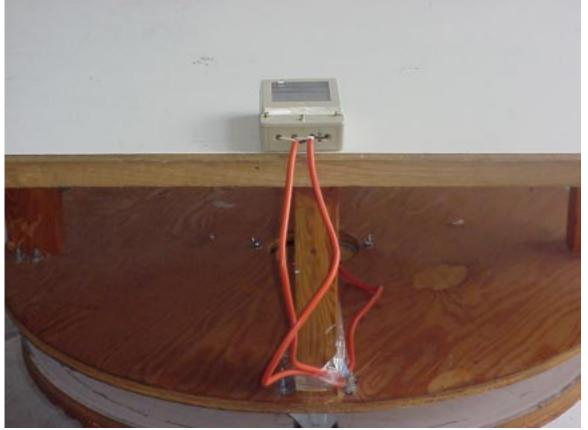
Worst Case Radiated Emissions Test Configuration
