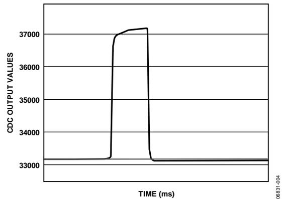
Figure 3. 8 mm Diameter Button Response
