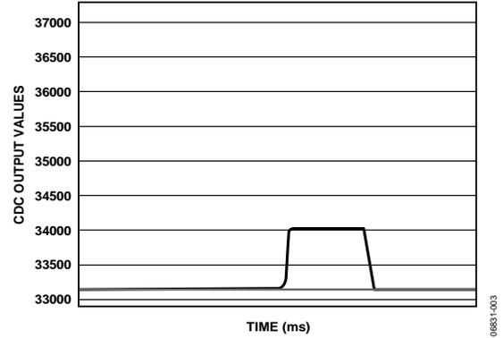
Figure 2. 4 mm Diameter Button Response
