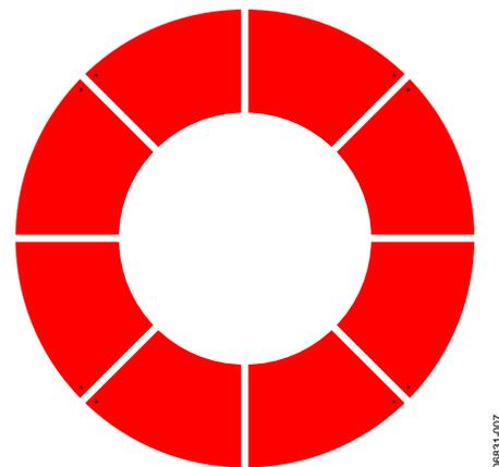
Figure 6. Scroll Wheel Sensor Layout
