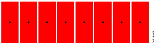
Figure 5. Discrete Slider Sensor Layout
