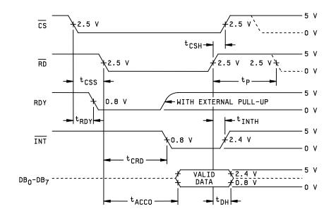
WR-RD mode stand-alone operation,  $\overline{CS} = \overline{RD} = 0$
