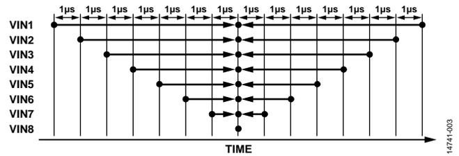
Figure 3. Time Averaged Samples Align with VIN8
