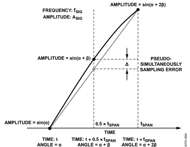
Figure 4. Determining Sampling Error
