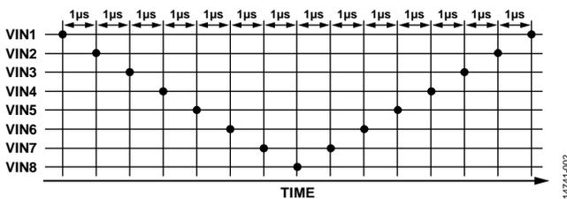
Figure 2. Analog Channel VINx Sampling Pattern
