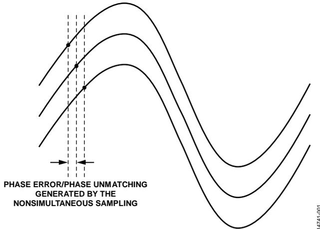
Figure 1. Phase Mismatch Due to Nonsimultaneous Sampling
