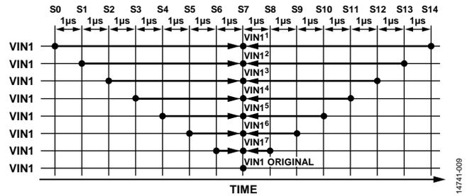
Figure 9. VIN1 Sample (S0 to S14)
