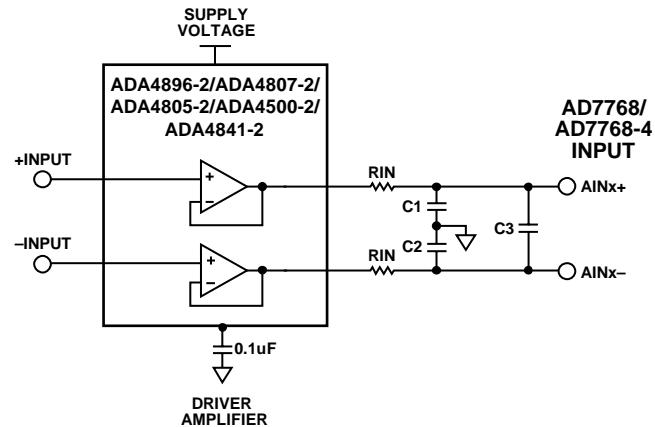
Figure 6. Typical Drive Amplifier Configuration
