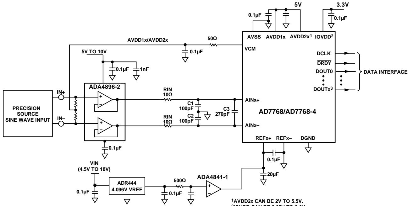
Figure 1. Typical Connection Diagram for the AD7768/AD7768-4 in Fast Power Mode, with the ADA4896-2 as the Driver Amplifier
