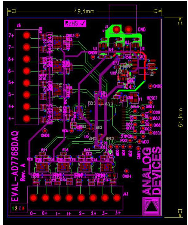
Figure 5. Example DAQ Footprint for the [AD7768/AD7768-4](#) and the [ADA4805-2](#)
