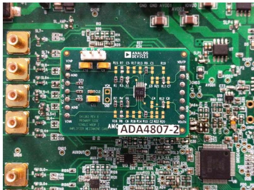
Figure 3. The ADA4807-2 AMC Setup on the EVAL-AD7768FMCZ
