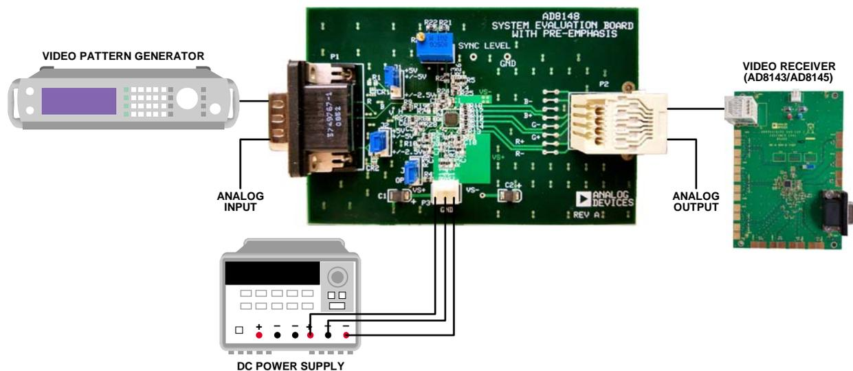
Figure 2. Typical Evaluation Setup
