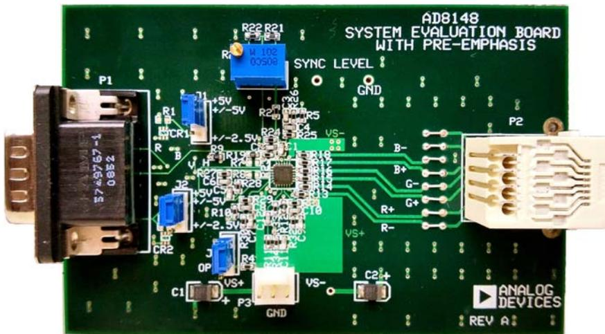
Figure 4. AD8147-EVALZ/AD8148-EVALZ Evaluation Board, Front Side
