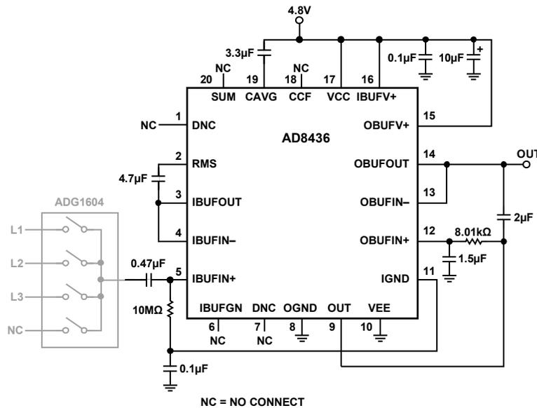
Figure 29. LFCSP [AD8436](#) of High Impedance Input and Precision Output Buffers Configured to Accommodate High Impedance Sources and a Two-Pole, Sallen-Key Low-Pass Output Filter
