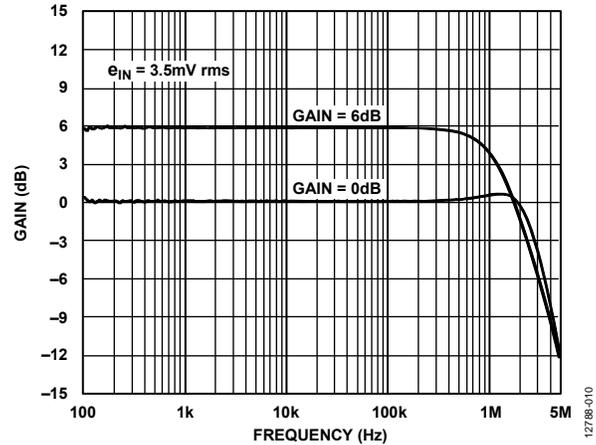
Figure 10. AD8436 FET Input Buffer Small Signal Bandwidth for Both Internal Gain Options
