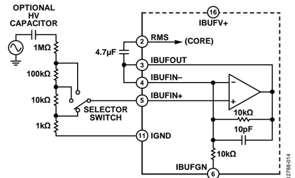
Figure 14. Range Switching for the LFCSF AD8436 FET Input Buffer
