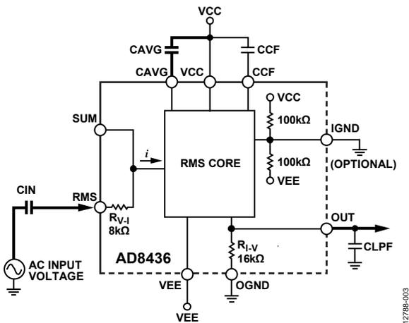
Figure 3. Minimum of Input/Output Connections (Emphasized Lines are the Signal Path)
