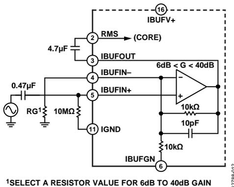
Figure 12. FET Input Buffer Configured for External Gain Adjustment for LFCSF
