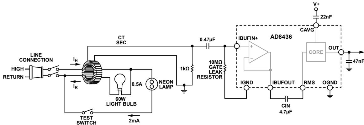
Figure 24. Ground Fault (Residual Current) Test Circuit with the AD8436 Configured as a Precision Full Wave Rectifier (Absolute Value Circuit)
