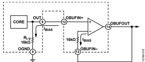
Figure 16. Precision DC Output Buffer Showing Cancellation of the Common-Mode Bias Current Component of  $V_{OS}$
