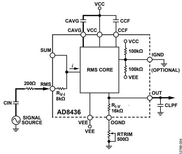
Figure 4. Basic AC-Coupled Calibration
