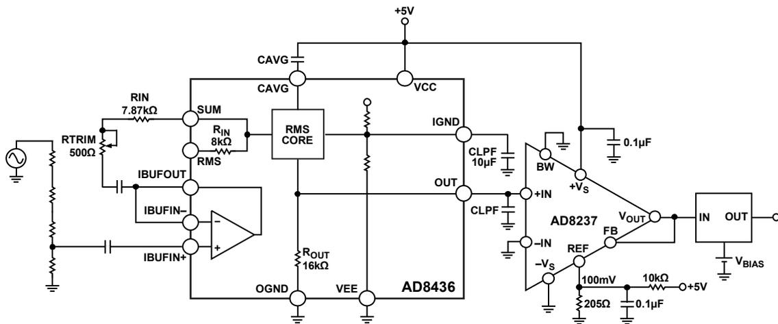
Figure 20. Schematic of AD8436 Configured for Single Supply and a Biased Output Load
