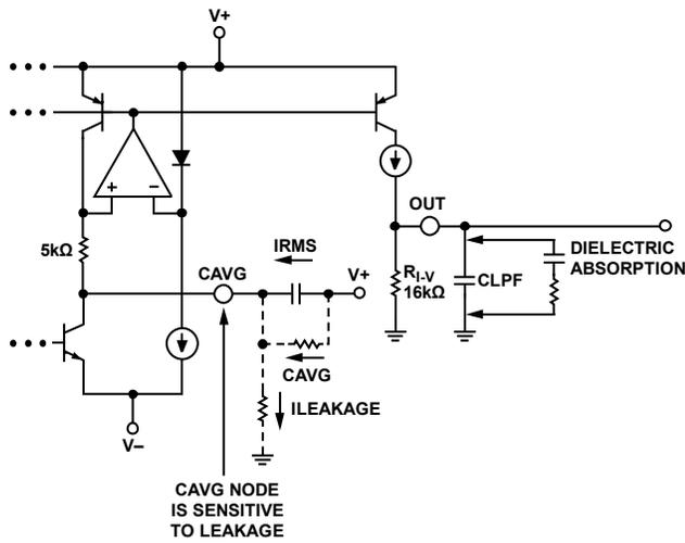
Figure 30. Capacitor and Leakage Errors
