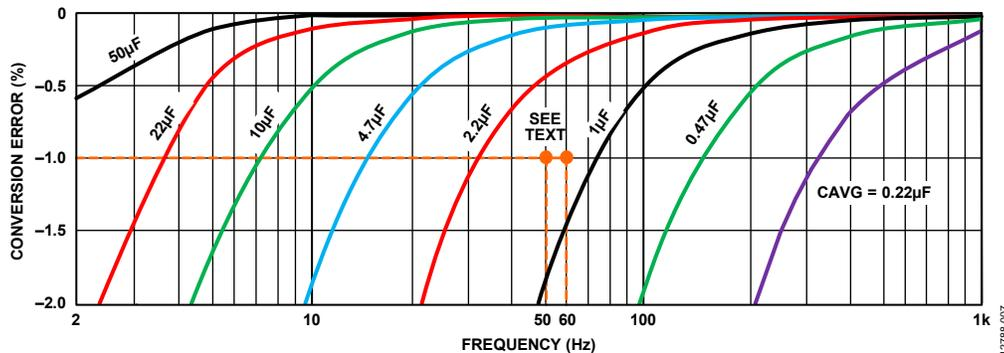
Figure 7. Conversion Error vs. Frequency for Various Values of CAVG (Method 1)
