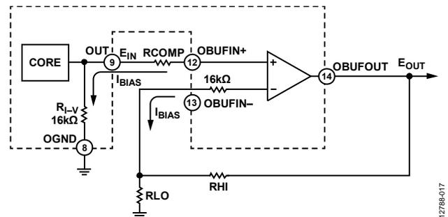
Figure 17. LFCSP AD8436 Precision DC Op Amp Buffer Configured for Greater than Unity Gain
