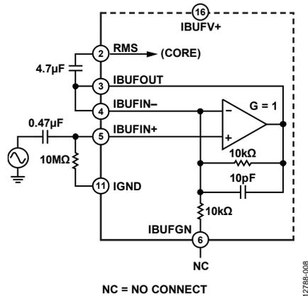
Figure 8. AC-Coupled High Impedance Input Buffer Configured for Unity Gain for LFCSP
