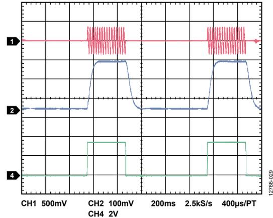
Figure 28. Timing Measurements of the [AD8436](#) Configured for 3-Phase Conversion; Trace 1: Input Burst—16 Cycles, 20 ms per Cycle, 1 sec Period; Trace 2: Output; Trace 3: Timing Reference—Burst Gate (Sync Output of Function Generator)
