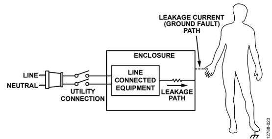
Figure 22. Human Hazard Caused by a Ground Fault Current Path
