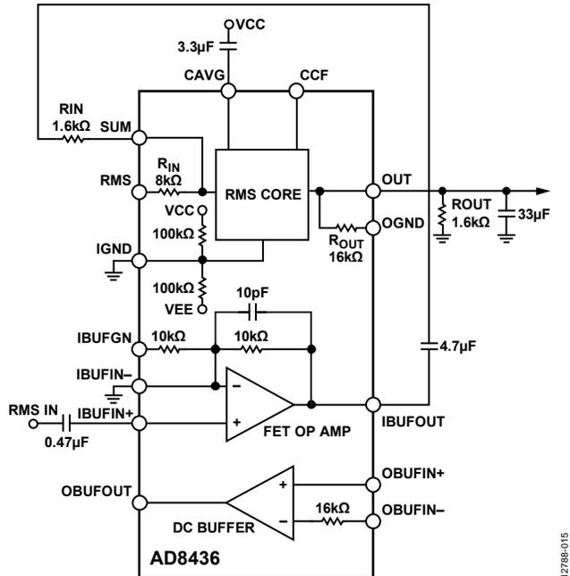
Figure 15. AD8436 Optimized for Low Voltage Input to Enhance the Turn On
