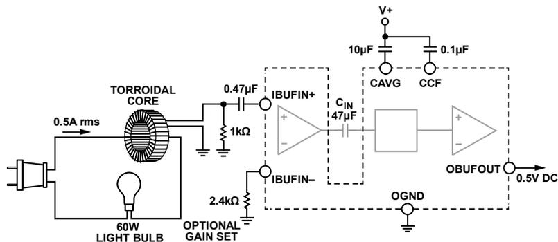
Figure 23. Block Diagram of [AD8436](#) Current Transformer Configuration
