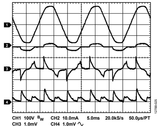
Figure 25. Simulated GFI Experiment Test Circuit Waveforms (see Figure 24); Trace 1: Neon Lamp Voltage; Trace 2: Neon Lamp Current; Trace 3: Current Transformer Load Resistor Waveform; Trace 4: Output of AD8436 Applied to Comparator Input
