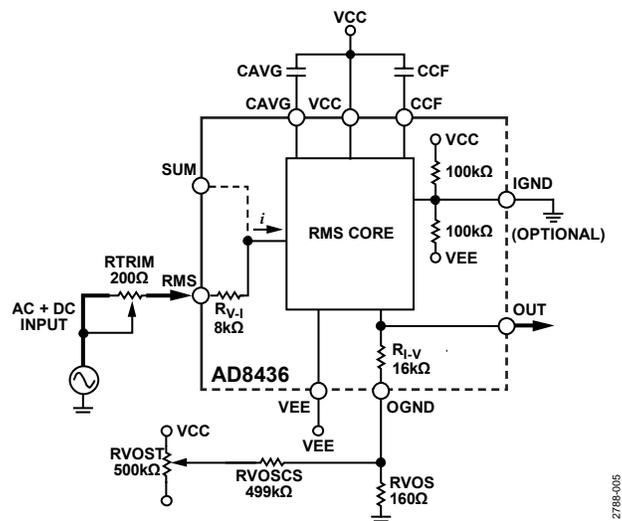
Figure 5. Optional Input Connections for AC + DC Signals, Including Offset Correction and Trim (V<sub>CC</sub> = +5 V, V<sub>EE</sub> = -5 V)
