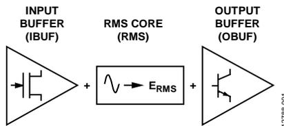
Figure 1. The Three Independent Circuits
