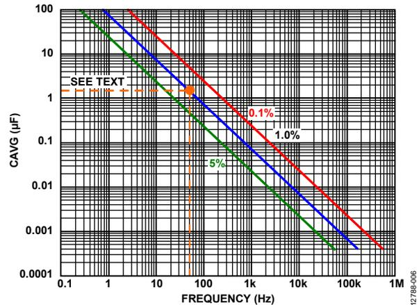
Figure 6. CAVG vs. Frequency for Three Error Values (Method 3)
