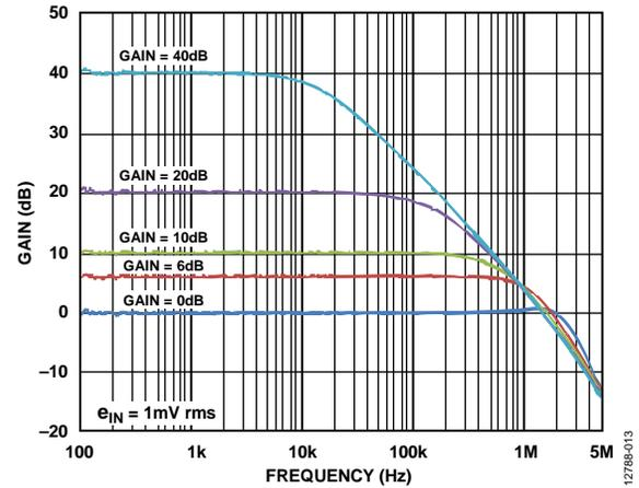
Figure 13. Gain and Bandwidth Options for the FET Input Buffer for Five Values of Gain
