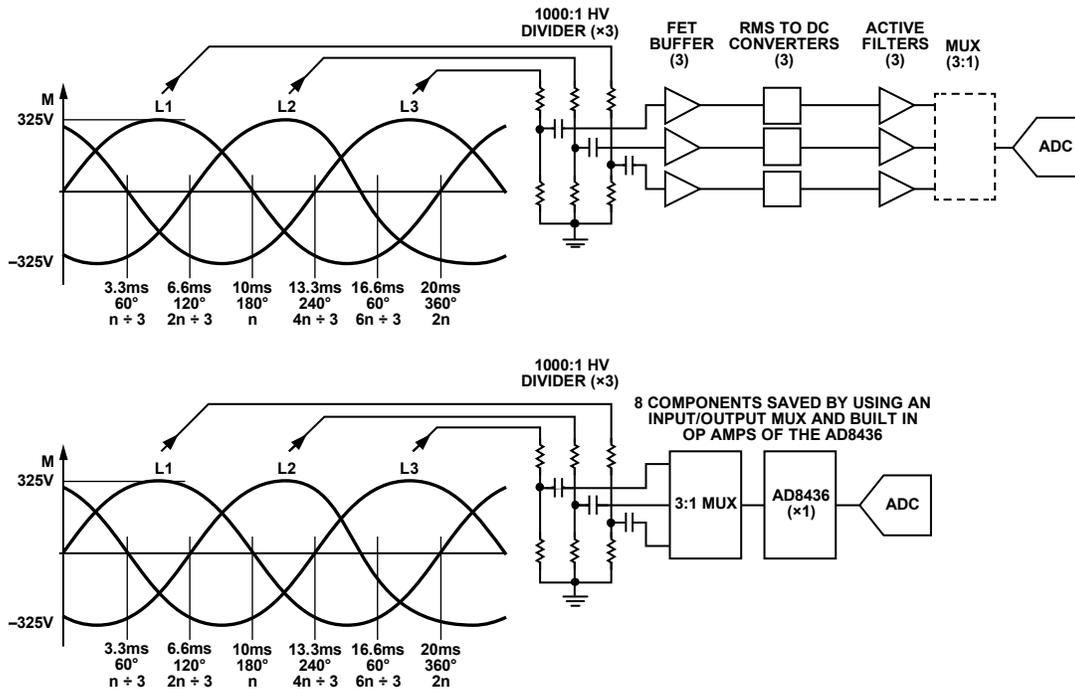
Figure 27. Comparison of Two Methods of Measuring 3-Phase Utility RMS Voltages Using the AD8436
