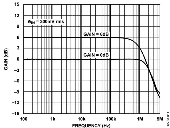
Figure 11. AD8436 FET Input Buffer Large Signal Bandwidth for Gain = 0 dB and 6 dB
