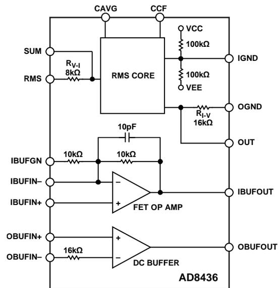
Figure 2. Functional Block Diagram of the **AD8436** RMS to DC Converter
