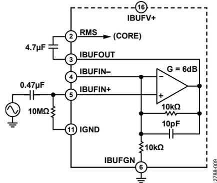
Figure 9. AC-Coupled High Impedance Input Amplifier Configured for G = 6 dB for LFCSP
