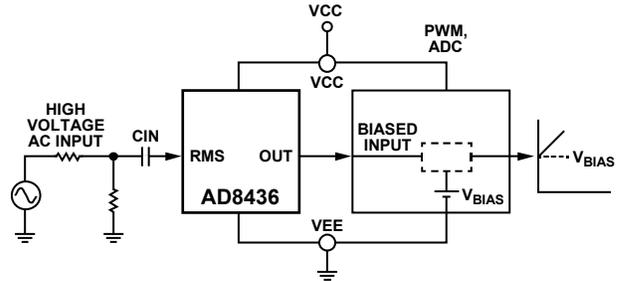
Figure 19. Block Diagram of the AD8436 Driving an External Device Requiring a Fixed DC Input Bias
