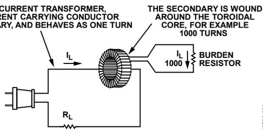
Figure 21. Toroidal Current Transformer Schematic
