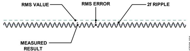
Figure 31. AD8436 Output Components
