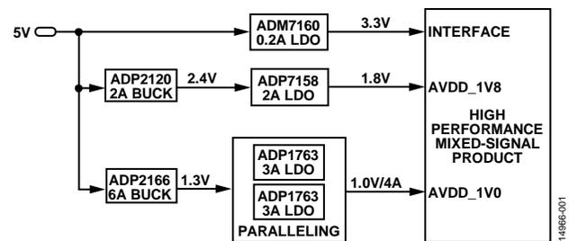
Figure 1. Power Diagram of Mixed-Signal Product
