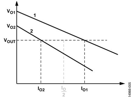
Figure 5. Passive Paralleling Load Regulation
