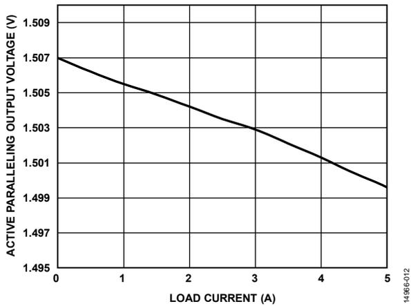
Figure 12. Active Paralleling Output Voltage vs. Load Current
