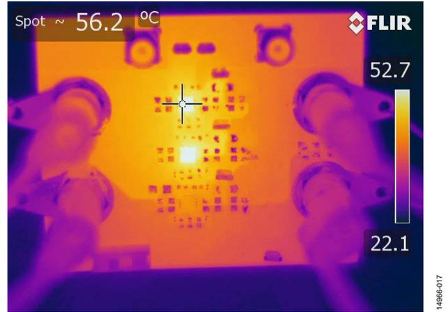
Figure 17. Thermal Test of Passive Paralleling
