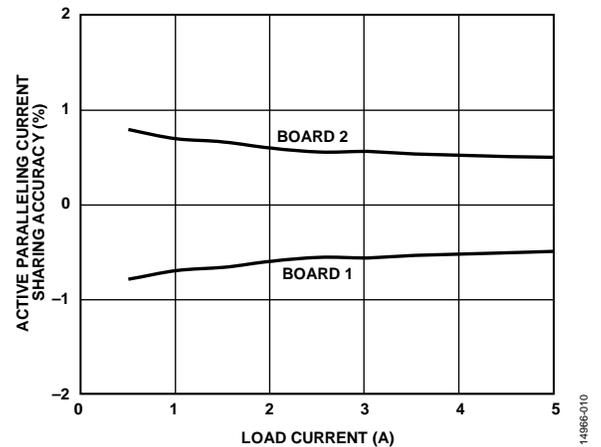
Figure 10. Active Paralleling Current Sharing Accuracy vs. Load Current
