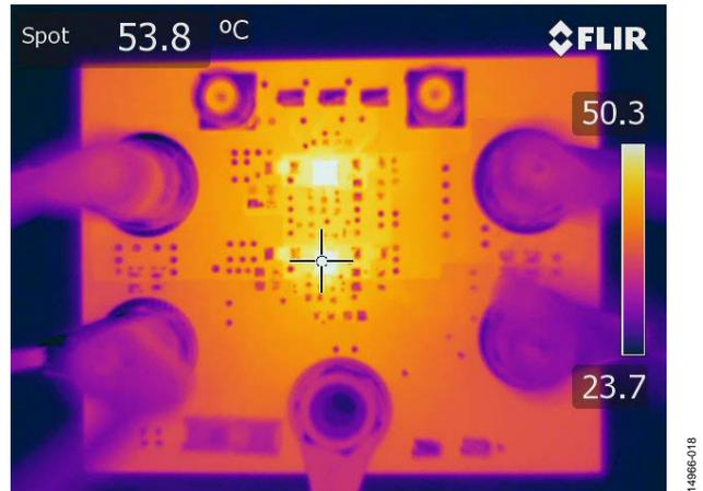
Figure 18. Thermal Test of Active Paralleling
