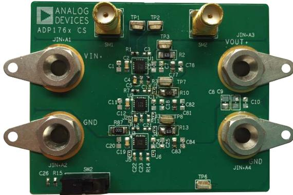
Figure 7. Passive Current Sharing Evaluation Board
