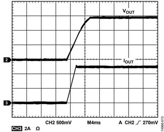
Figure 13. Soft Start of Passive Paralleling
