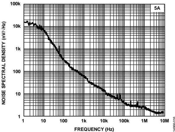
Figure 16. NSD vs. Frequency at  $V_{IN} = 1.8\text{ V}$ ,  $I_O = 5\text{ A}$  NSD of Active Paralleling
