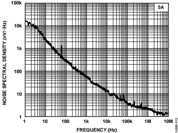
Figure 15. Noise Spectral Density (NSD) vs. Frequency at  $V_{IN} = 1.8\text{ V}$ ,  $I_O = 5\text{ A}$  NSD of Passive Paralleling
