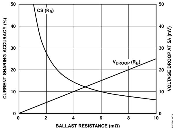
Figure 4. Current Sharing (CS) Accuracy and Voltage Droop vs. Ballast Resistance
