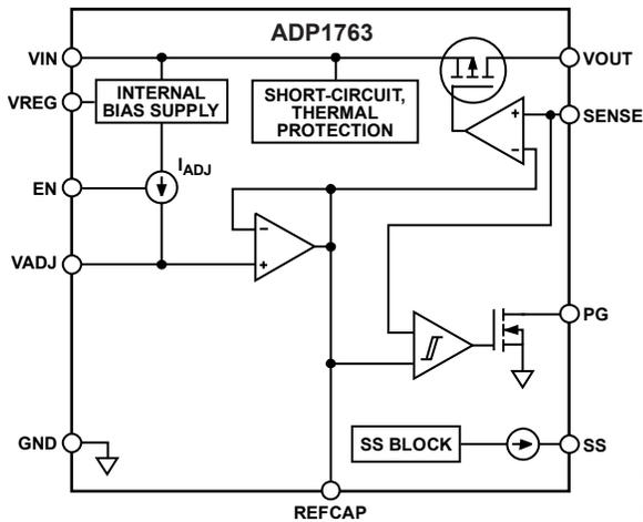
Figure 2. ADP1763 Internal Block Diagram
