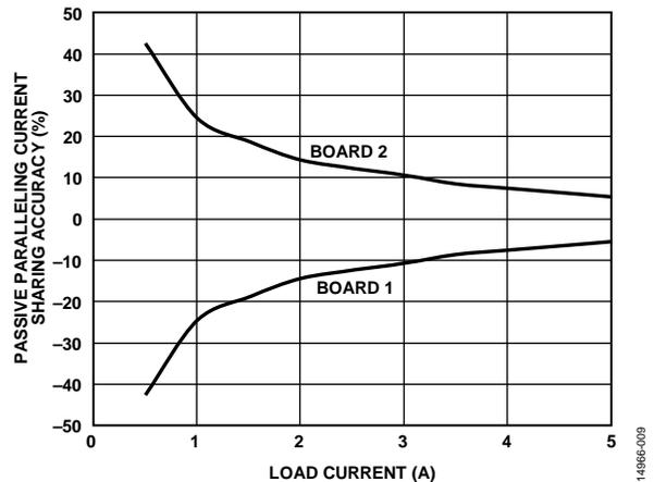
Figure 9. Passive Paralleling Current Sharing Accuracy vs. Load Current
