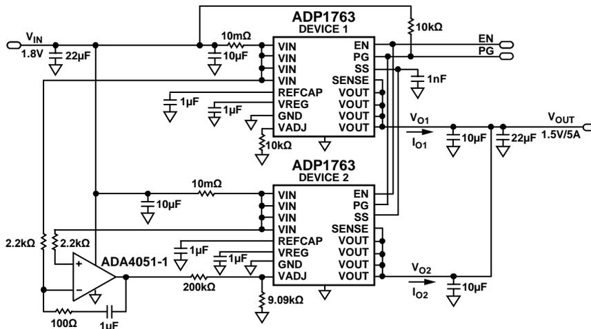
Figure 6. Active Paralleling the Two ADP1763 Devices
