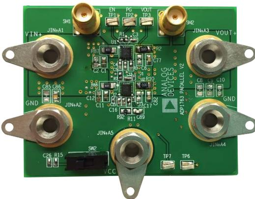
Figure 8. Active Current Sharing Evaluation Board
