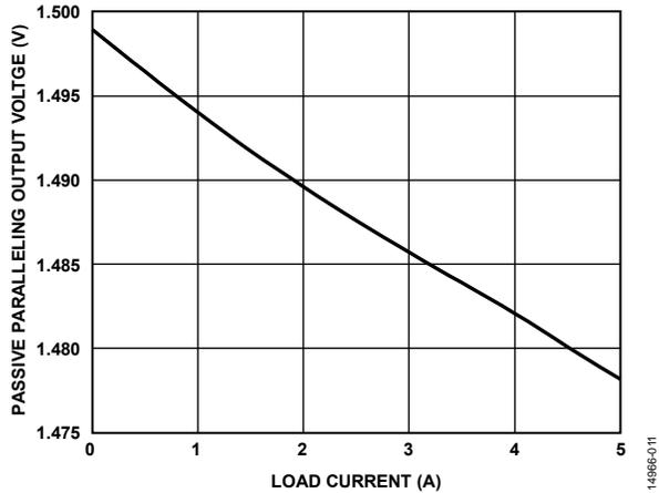
Figure 11. Passive Paralleling Output Voltage vs. Load Current
