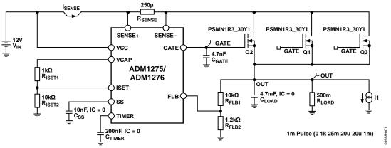
Figure 2. ADM1275/ADM1276 Simulation Model Schematic
