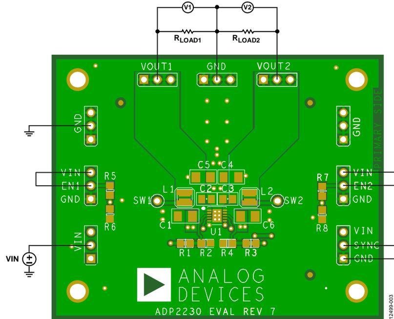
Figure 3. Output Voltage Measurement Setup
