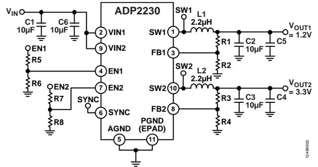
Figure 2. ADP2230 Evaluation Board Schematic
