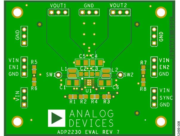
Figure 8. PCB Layout, Top
