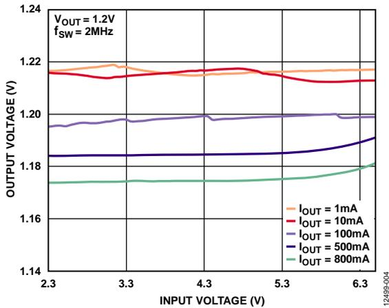
Figure 4. Line Regulation,  $V_{OUT} = 1.2\text{ V}$ , Different Loads
