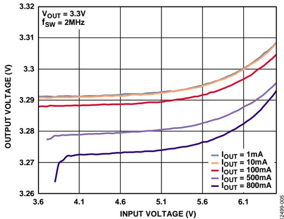
Figure 5. Line Regulation,  $V_{OUT} = 3.3\text{ V}$ , Different Loads
