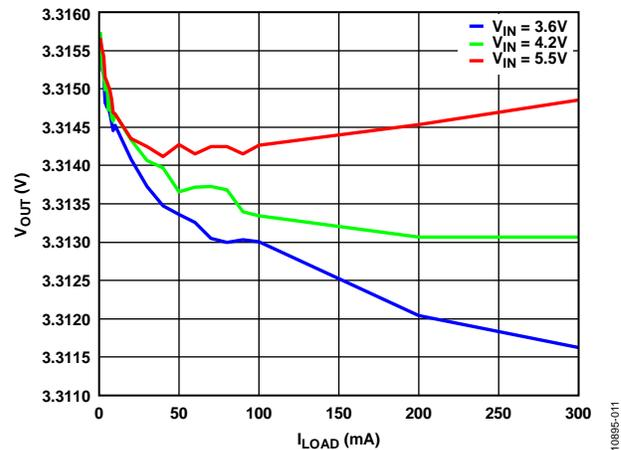
Figure 14.  $V_{OUT}$  vs.  $I_{LOAD}$  LDO Load Regulation
