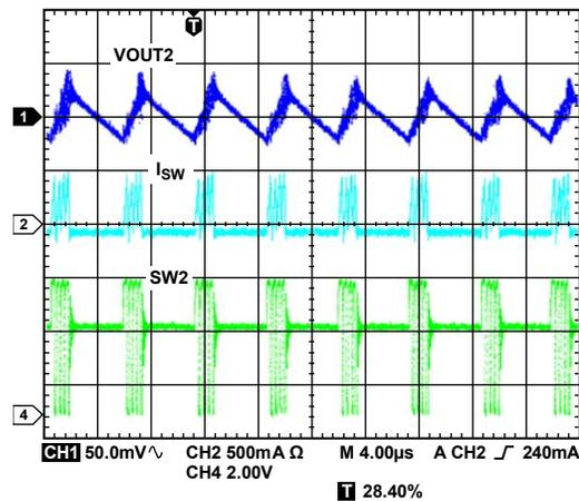
Figure 5. Typical Waveforms, V<sub>OUT2</sub> = 3.3 V, I<sub>OUT2</sub> = 30 mA, PSM Mode
