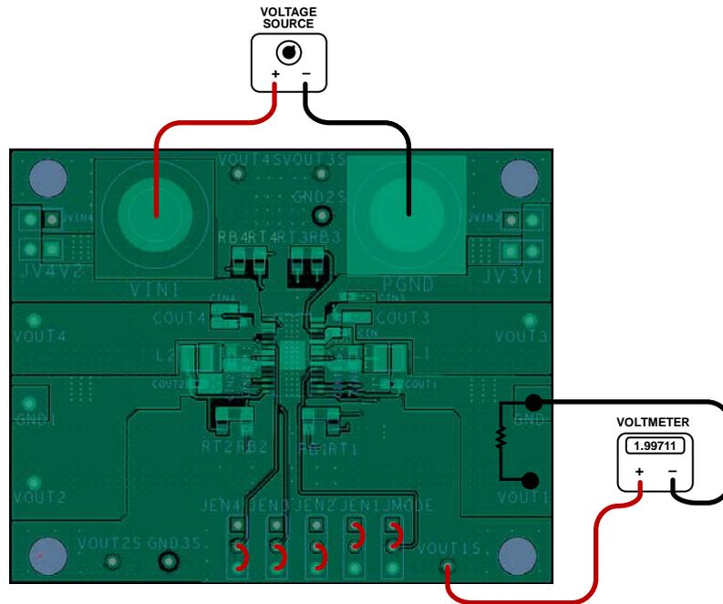
Figure 16. Output Voltage Measurement
