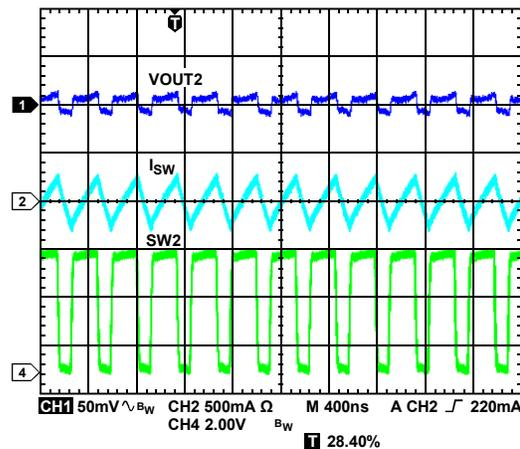
Figure 6. Typical Waveforms, V<sub>OUT2</sub> = 3.3 V, I<sub>OUT2</sub> = 30 mA, PWM Mode
