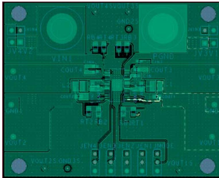
Figure 20. Top Layer, Recommended Layout for ADP5034 TSSOP
