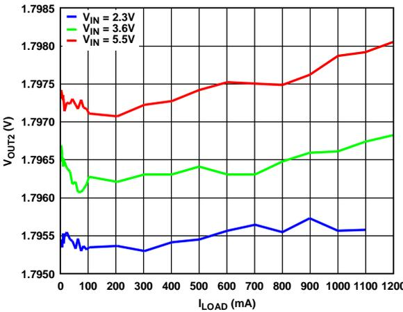
Figure 8. Buck Load Regulation,  $V_{OUT2} = 1.8\text{ V}$
