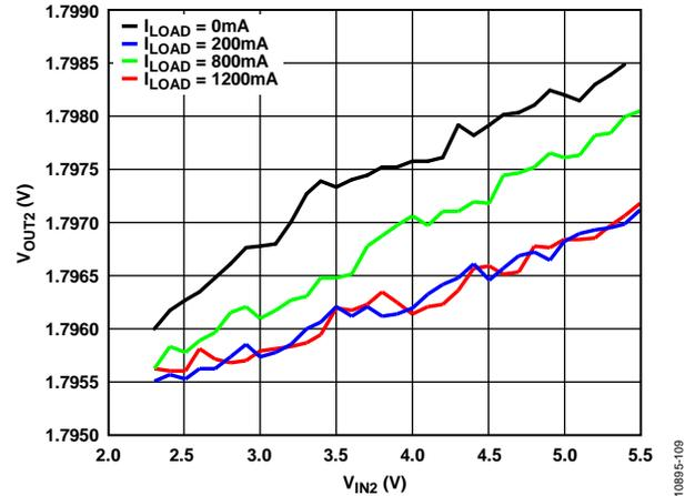
Figure 10. Buck Regulator Line Regulation,  $V_{OUT2} = 1.8\text{ V}$
