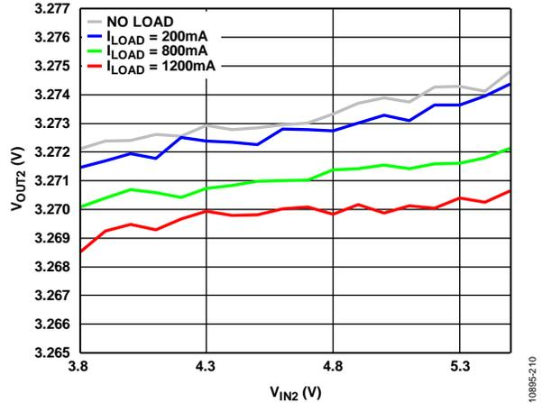
Figure 9. Buck Regulator Line Regulation,  $V_{OUT2} = 3.3\text{ V}$
