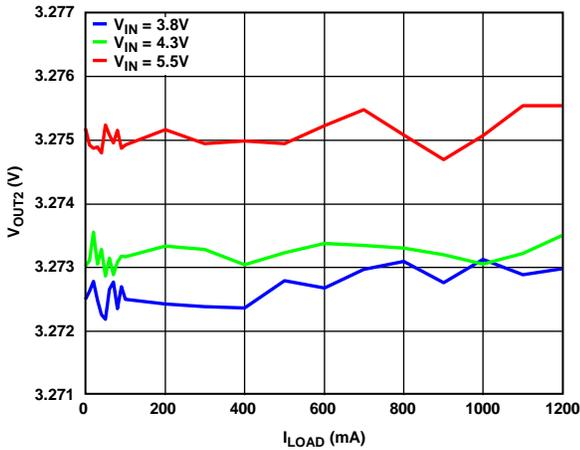
Figure 7. Buck Load Regulation,  $V_{OUT2} = 3.3\text{ V}$
