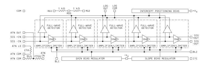
FIGURE 2. Block diagram.
