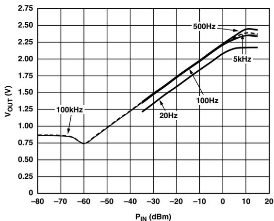
Figure 13. AD8307 Transfer Function for  $C_C = 100 \mu F$
