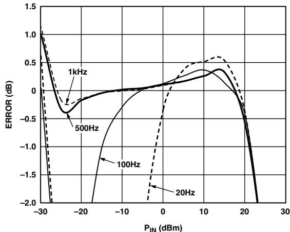
Figure 56. AD8302 Gain Conformance for  $C_C = 100 \mu F$
