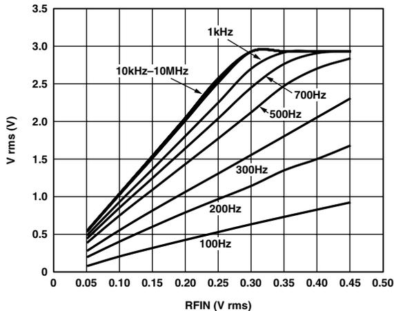
Figure 31. AD8361 Transfer Function for  $C_C = 1 \mu F$
