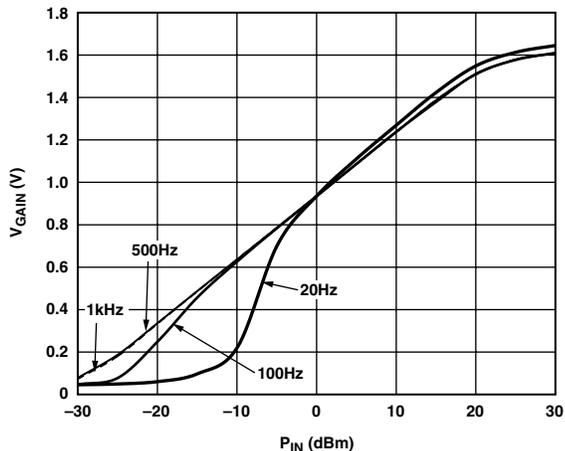
Figure 54. AD8302 Gain Output for  $C_C = 100 \mu F$
