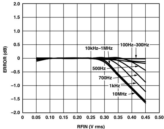
Figure 34. AD8361 Law Conformance for  $C_C = 1 \mu F$
