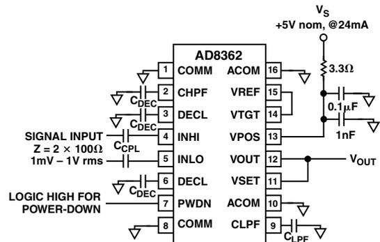
*Figure 37. AD8362 Typical Connections for Measurement Mode*
