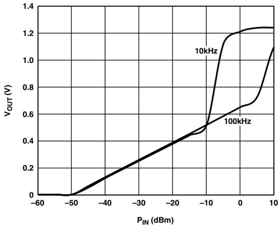
Figure 40. AD8362 Transfer Function for  $C_C = 0.1 \mu F$
