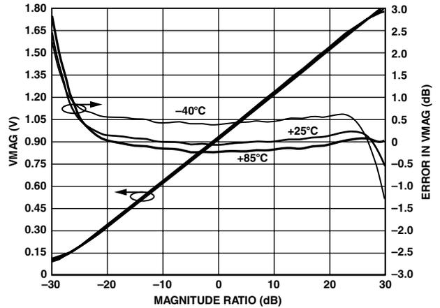
Figure 47. AD8302 Log Slope and Error at 100 MHz
