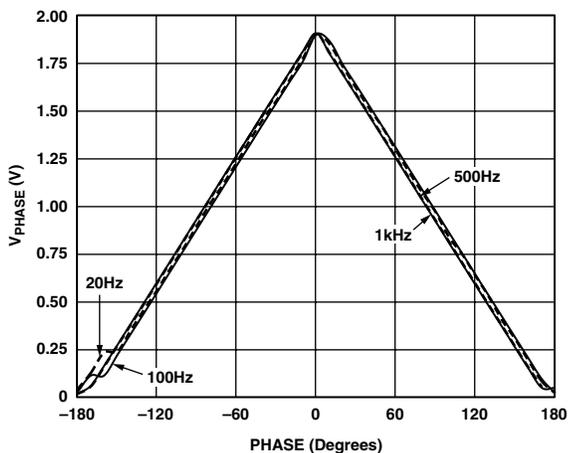
Figure 55. AD8302 Phase Output for  $C_C = 100 \mu F$
