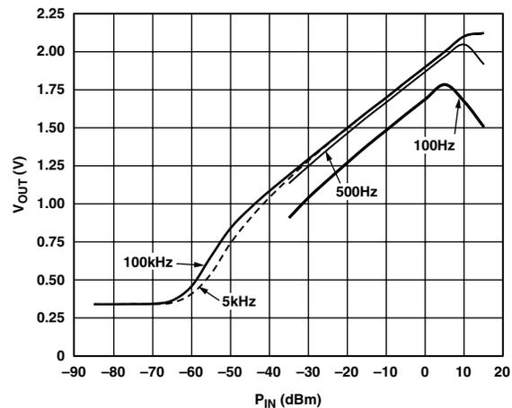
Figure 20. AD8309 Transfer Function at Low Frequencies
