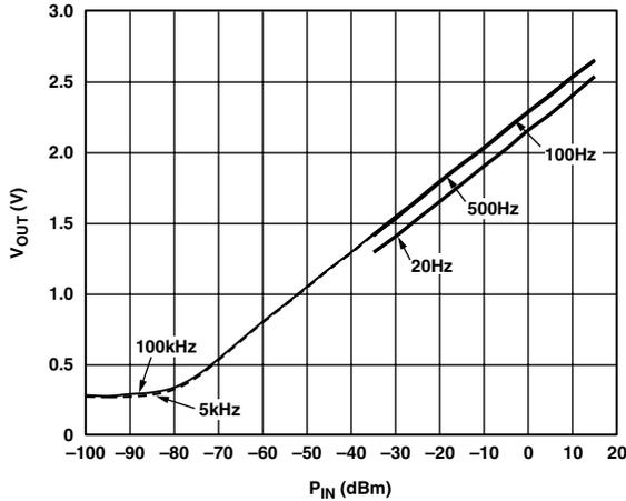
Figure 25. AD8310 Log Slope at Low Frequencies
