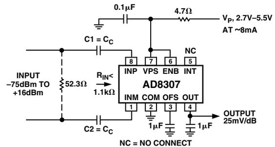
Figure 10. AD8307 Modifications for Low Frequency Operation
