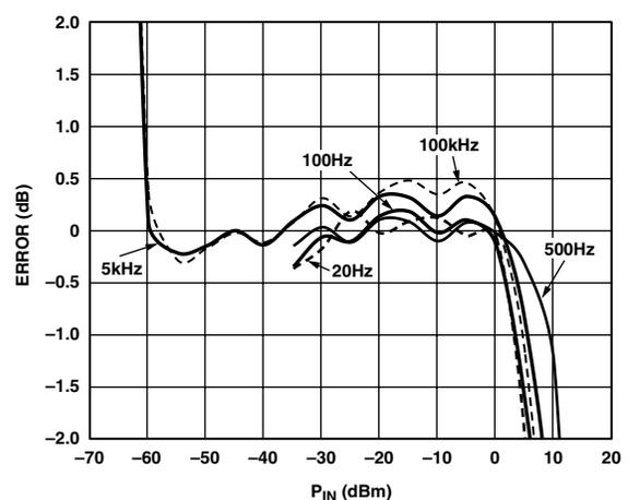
Figure 45. AD8362 Law Conformance for  $C_C = 100 \mu F$
