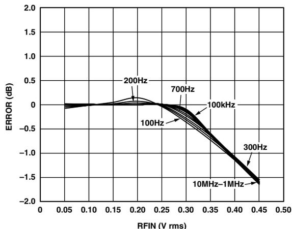
Figure 36. AD8361 Law Conformance for  $C_C = 100 \mu F$
