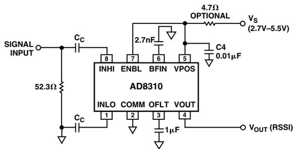
Figure 27. AD8310 Modifications for Low Frequency Operation
