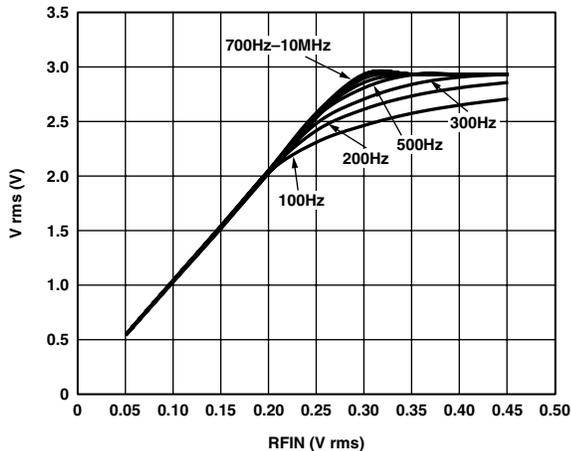
Figure 33. AD8361 Transfer Function for  $C_C = 100 \mu F$
