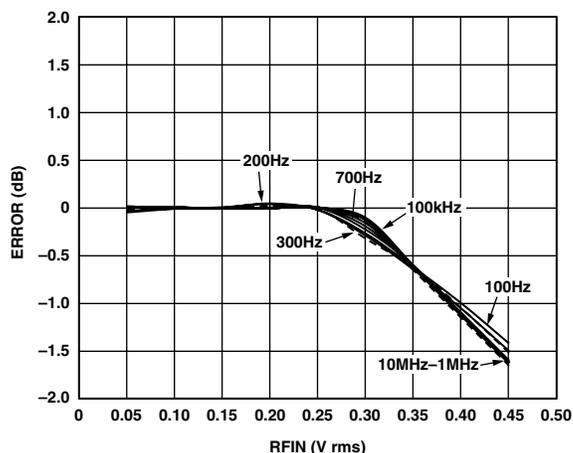
Figure 35. AD8361 Law Conformance for  $C_C = 10 \mu F$
