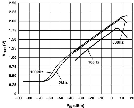
Figure 5. AD8306 Detector Transfer Function for Low Frequencies
