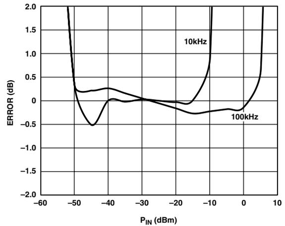
Figure 43. AD8362 Law Conformance for  $C_C = 0.1 \mu F$
