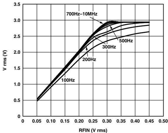
Figure 32. AD8361 Transfer Function for  $C_C = 10 \mu F$
