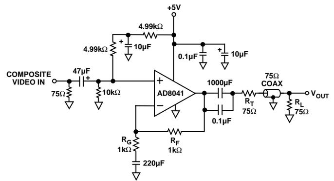
Figure 5. AC-Coupled Single-Supply Composite Video Line Driver
