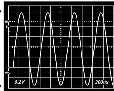
Figure 9. Output Signal Swing of Low Distortion Line Driver at 2 MHz
