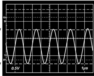
Figure 7. Output Signal Swing of Low Distortion Line Driver at 500 kHz
