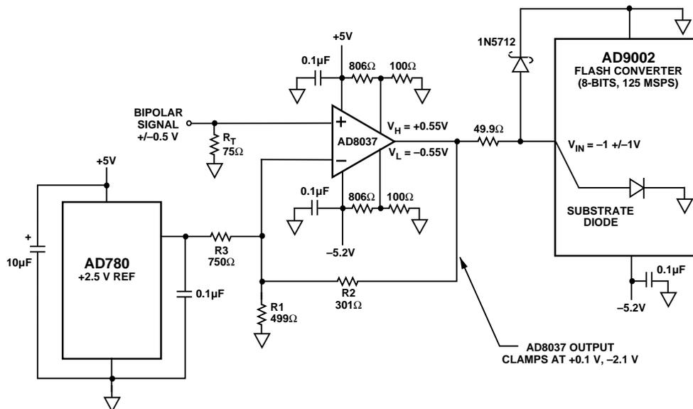
Figure 2. AD9002, 8-Bit, 125 MSPS Flash Converter
