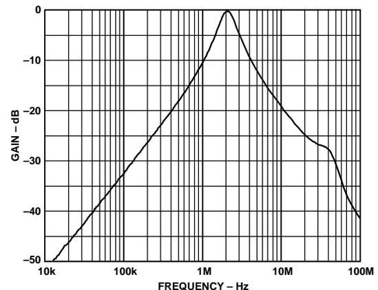
Figure 12. Frequency Response of Single-Supply 2 MHz Bandpass Filter
