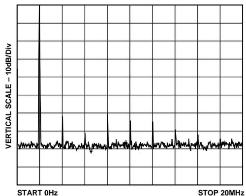
Figure 10. THD of Low Distortion Line Driver at 2 MHz
