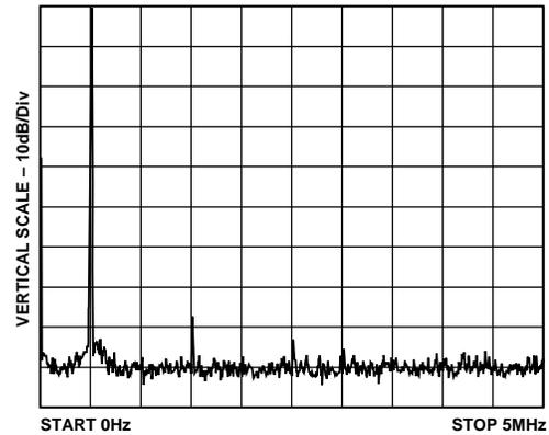
Figure 8. THD of Low Distortion Line Driver at 500 kHz
