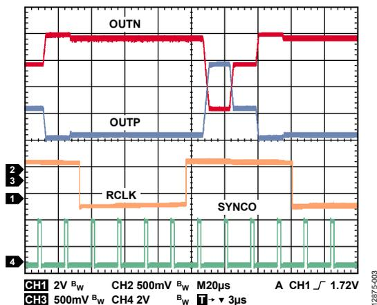
Figure 3. Expected RCLK\_OUT, VOP, VON, and SYNC\_OUT Waveforms
