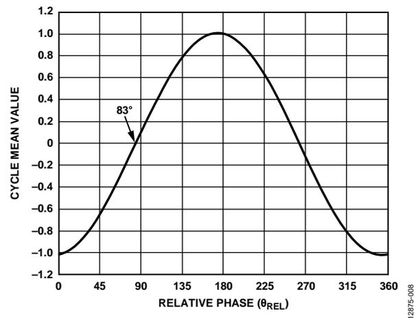
Figure 8. Phase Transfer Function with Phase Delay of 83°, 1 V rms Input
