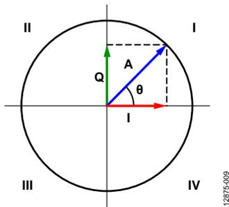
Figure 9. Rectangular and Polar Representation of a Signal
