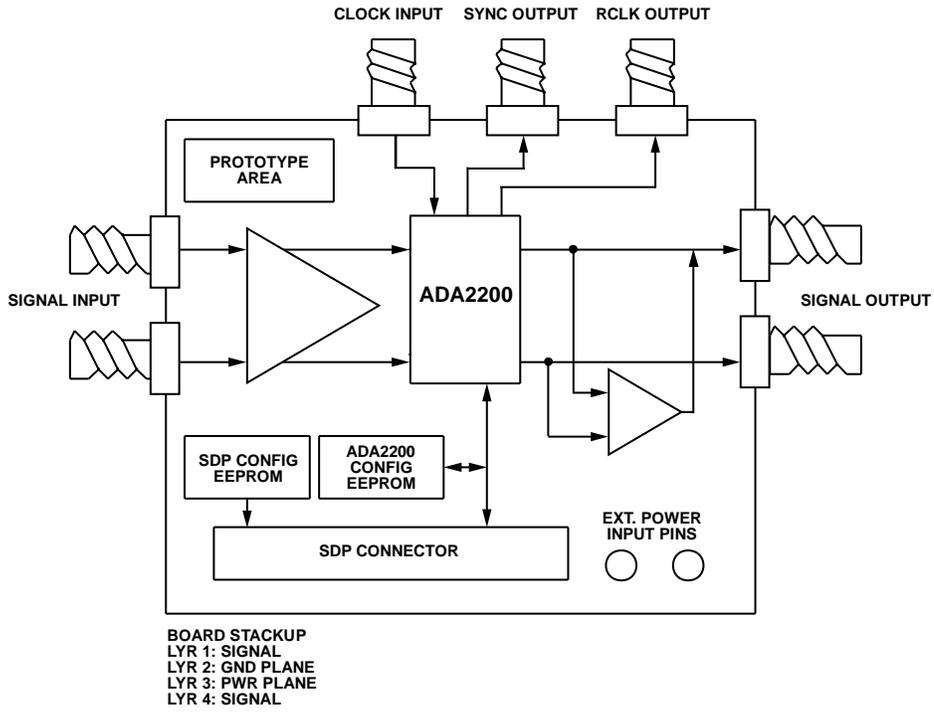
Figure 10. Evaluation Board Block Diagram
