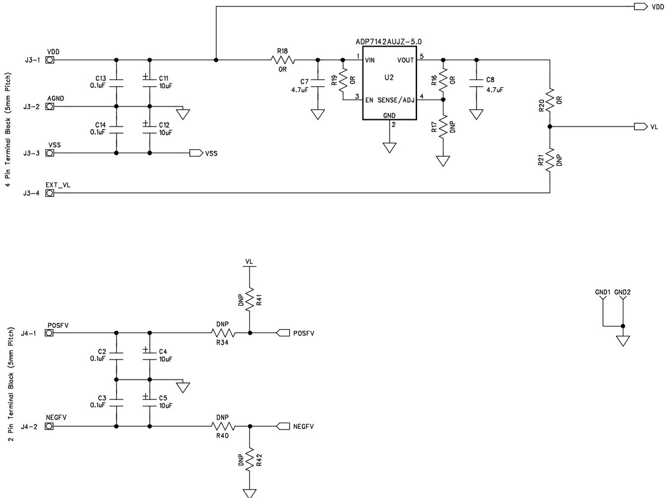
Figure 5. ADG5248F Evaluation Board Schematic (Part 3)
