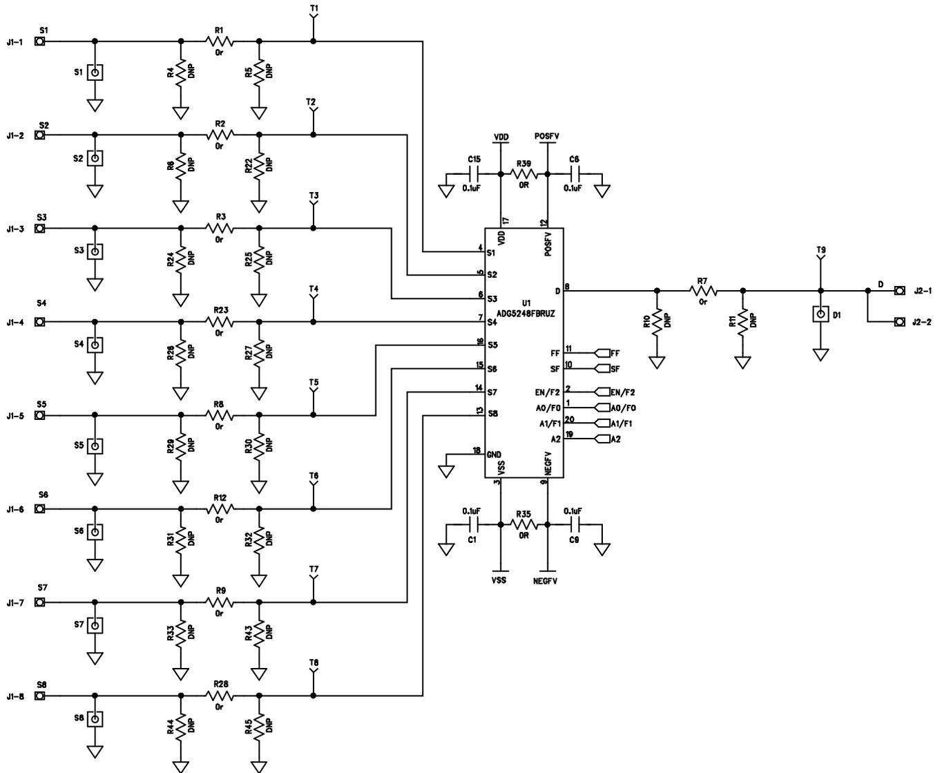
Figure 3. ADG5248F Evaluation Board Schematic (Part 1)
