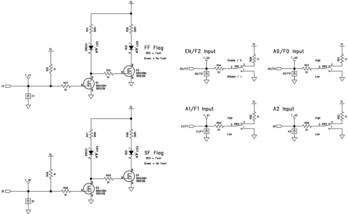
Figure 4. ADG5248F Evaluation Board Schematic (Part 2)
