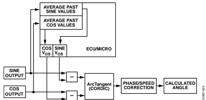
Figure 22. Single Point Calibration Operating Flow Chart
