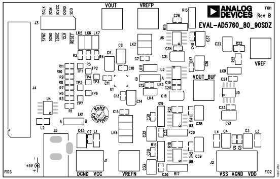
Figure 12. Component Placement Schematic
