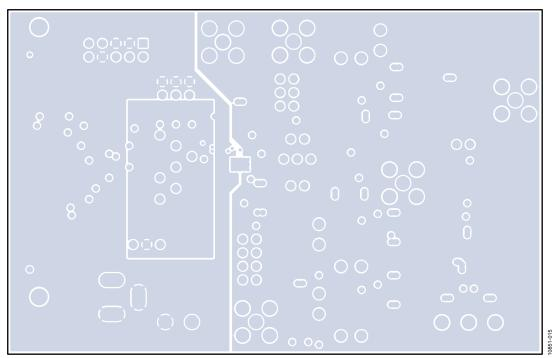
Figure 15. Inner Second PCB Layer Schematic
