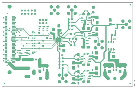
Figure 13. Top Printed Circuit Board (PCB) Layer Schematic
