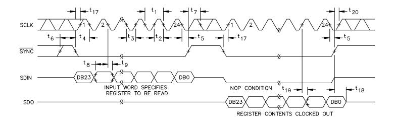
FIGURE 4. Readback mode timing diagram.
