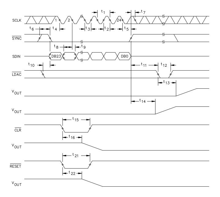
FIGURE 3. Write mode timing diagram.
