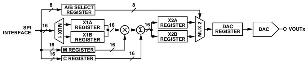
Figure 1. Functional Block Diagram of a Single Channel
