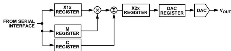
Figure 3. AD5362 Register Configuration
