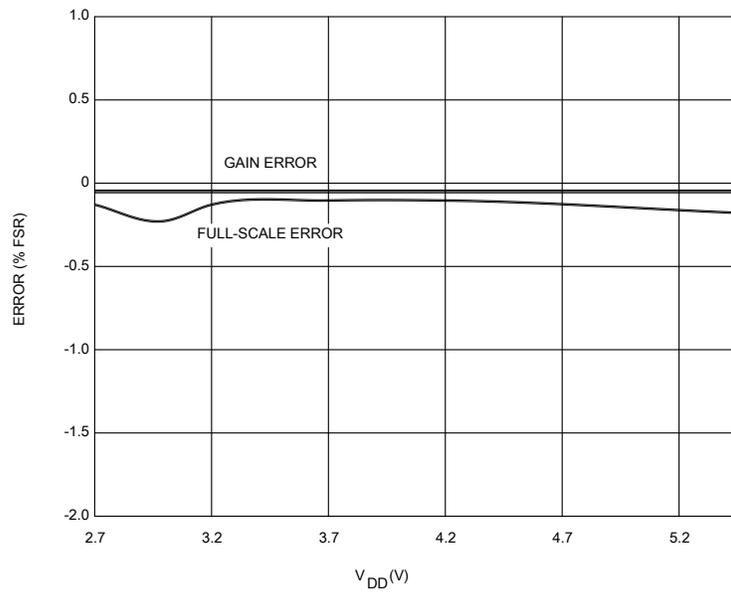
FIGURE 7. Gain error and Full scale error vs Supply voltage.
