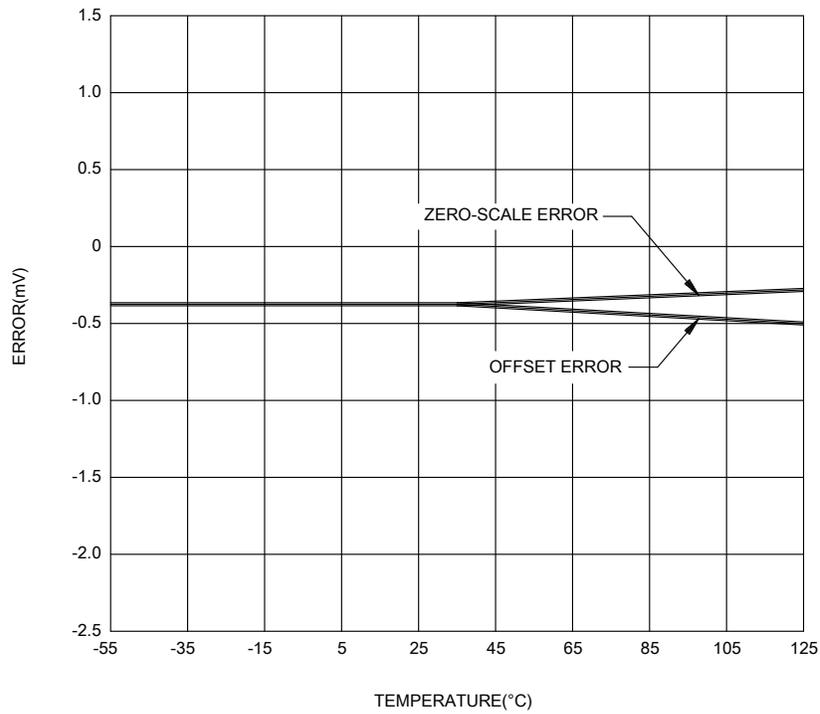
FIGURE 6. Zero scale error and Offset error vs Temperature.
