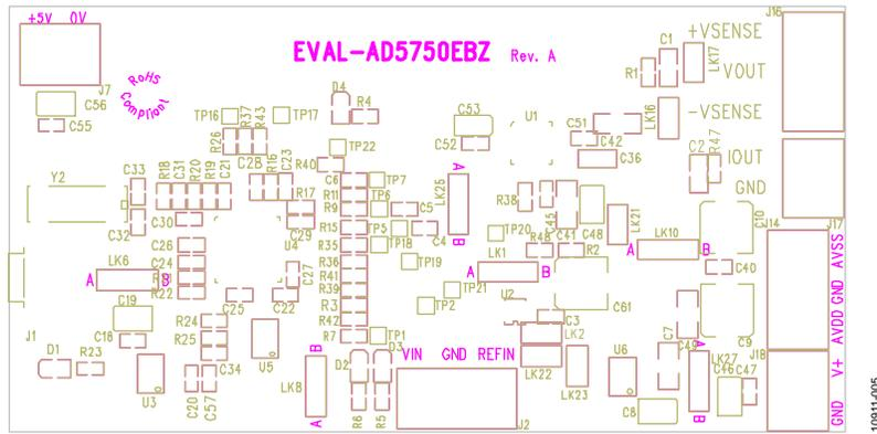
Figure 5. Component Placement
