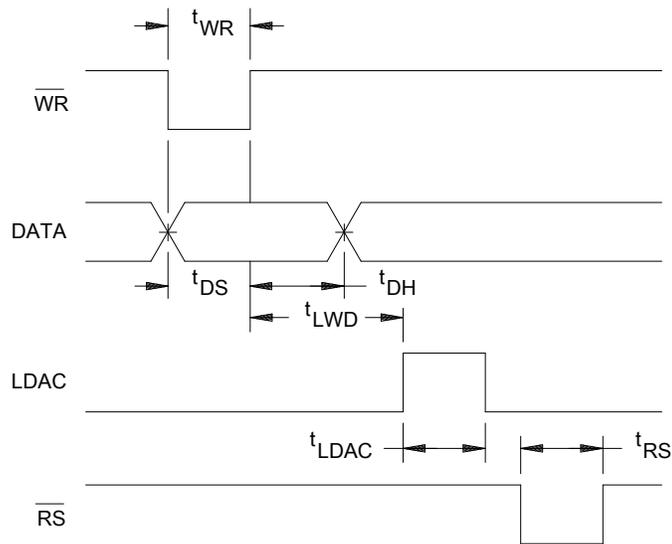
FIGURE 8. Timing diagram.
