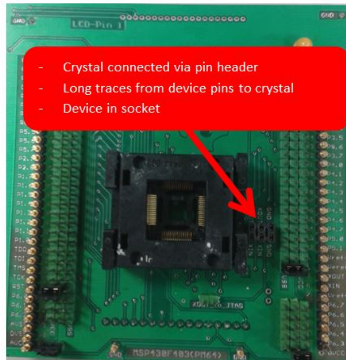
Figure 11. Nonoptimized PCB for General Test Purpose
