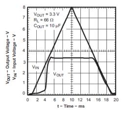
Figure 7. Power-up and Power-Down Behavior of TPS715A
