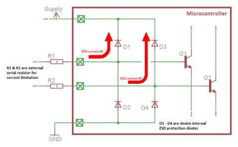
Figure 3. Principle Schematic of an I/O
