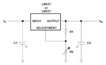
Figure 3. Adjustable Negative-Voltage Regulator
