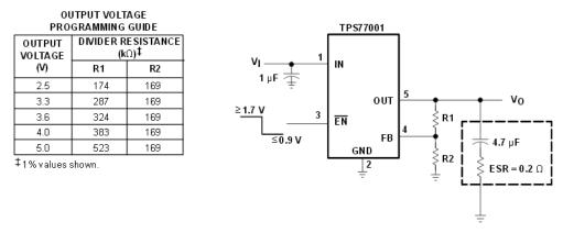
Figure 22. TPS77001 Adjustable LDO Regulator Programming
