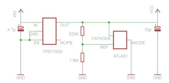
Figure 10. Schematic Example Using AT431
