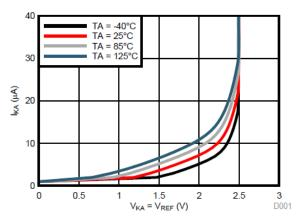
Figure 9. Cathode Current vs Cathode Voltage
