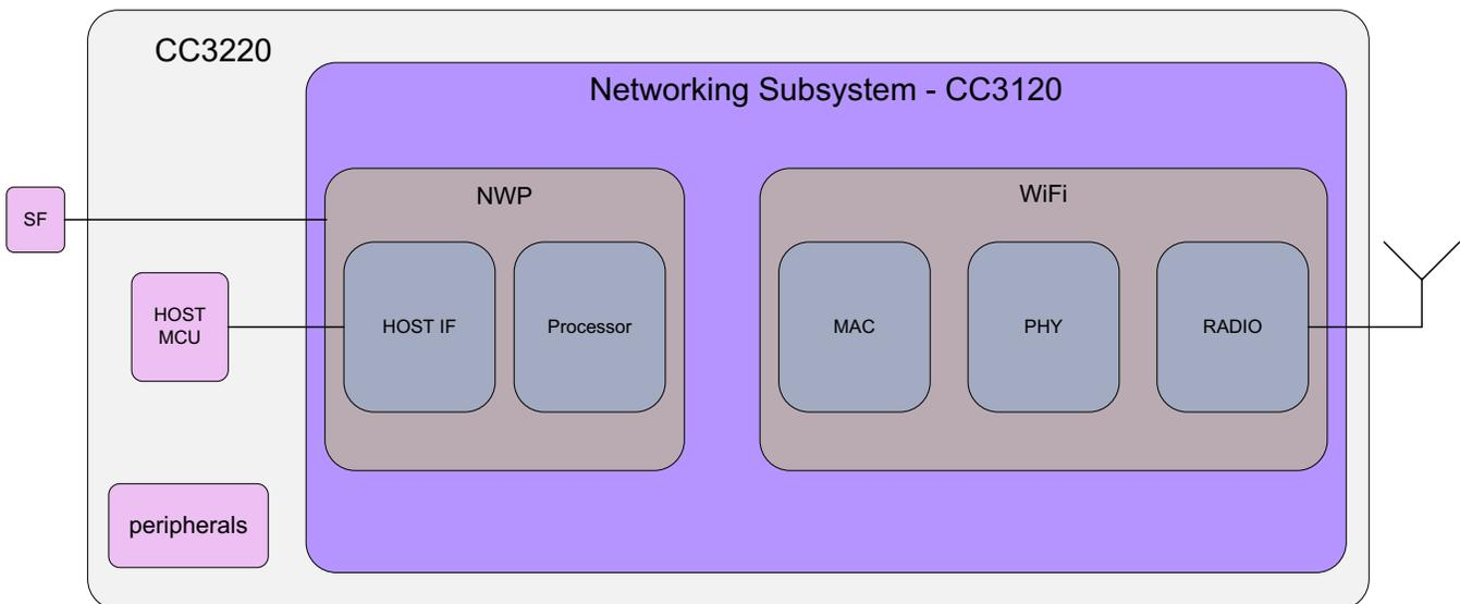
**Figure 1. CC3120, CC3220 Block Diagram**
