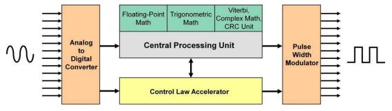
Figure 1. System Block Diagram With Accelerators
