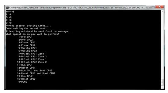
Figure 3. serial\_flash\_programmer Prompting for Next Command
