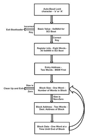
Figure 2. Bootloader Data Structure
