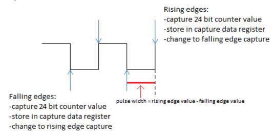
Figure 2: Timer Capture on a Waveform
